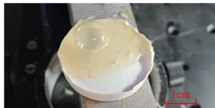
**Figure 4.** Physical image of acrylic AB adhesive bubble.
