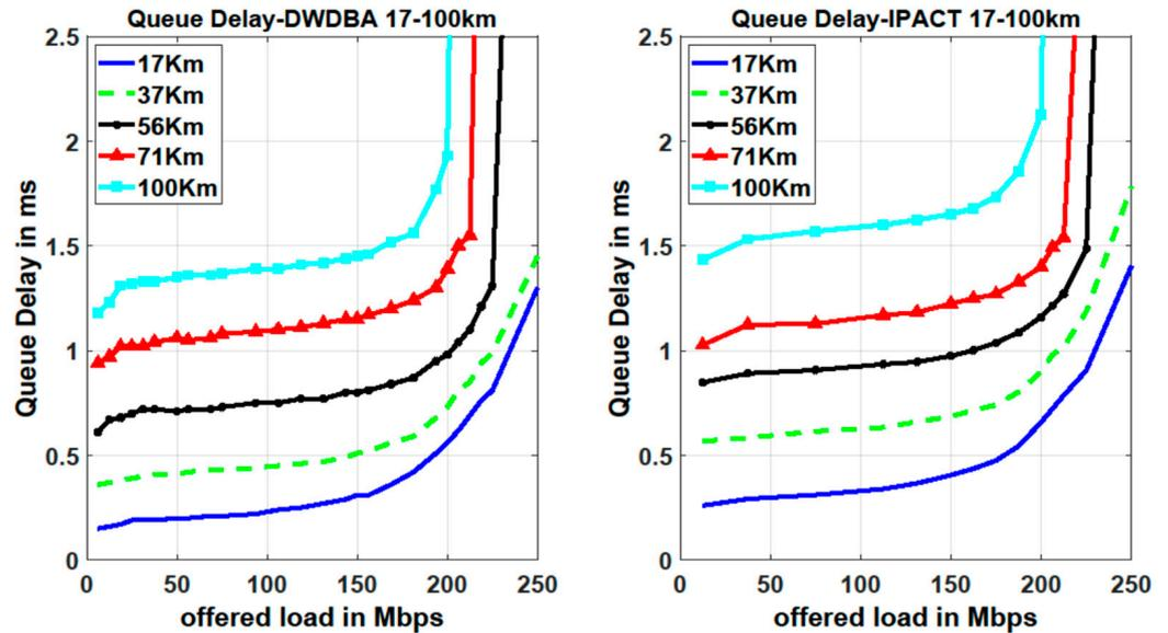
Figure 11. Queue delay for scenario 3 where the ONUs are placed between 17 km and 100 km from OLT for DWDBA (left) and IPACT (right).
