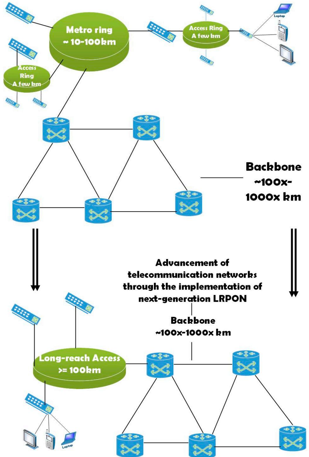
Figure 1. Evolution of LRPON (based on Figure 1 from [19]).
