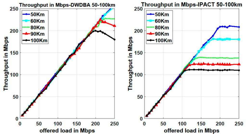
Figure 8. Throughput for scenario 4 where the ONUs are placed between 50 km and 100 km from OLT for DWDBA (left) and IPACT (right).
