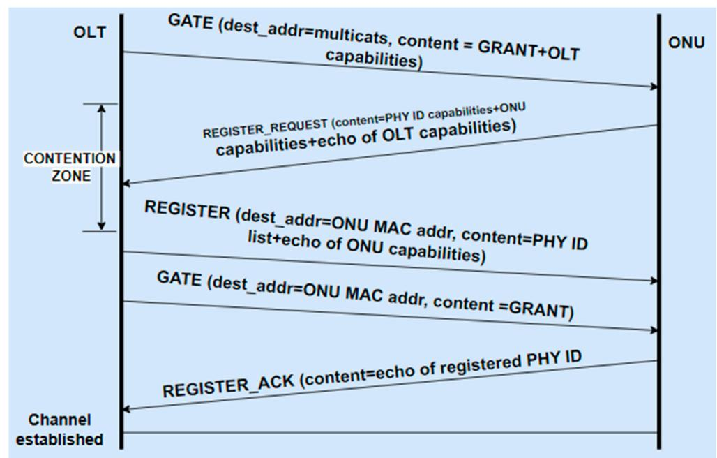
**Figure 2.** OLT and ONUs discovery and communication protocol. The contention zone is the period where multiple ONUs engage in competition to register with the OLT, ensuring collision avoidance.
