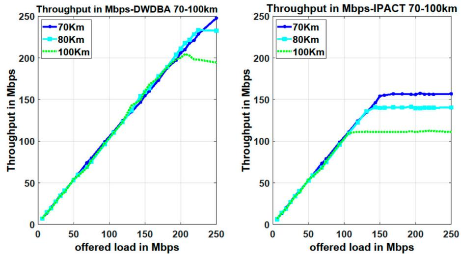
Figure 6. Throughput for scenario 2 where the ONUs are placed between 70 km and 100 km from OLT for DWDBA (left) and IPACT (right).
