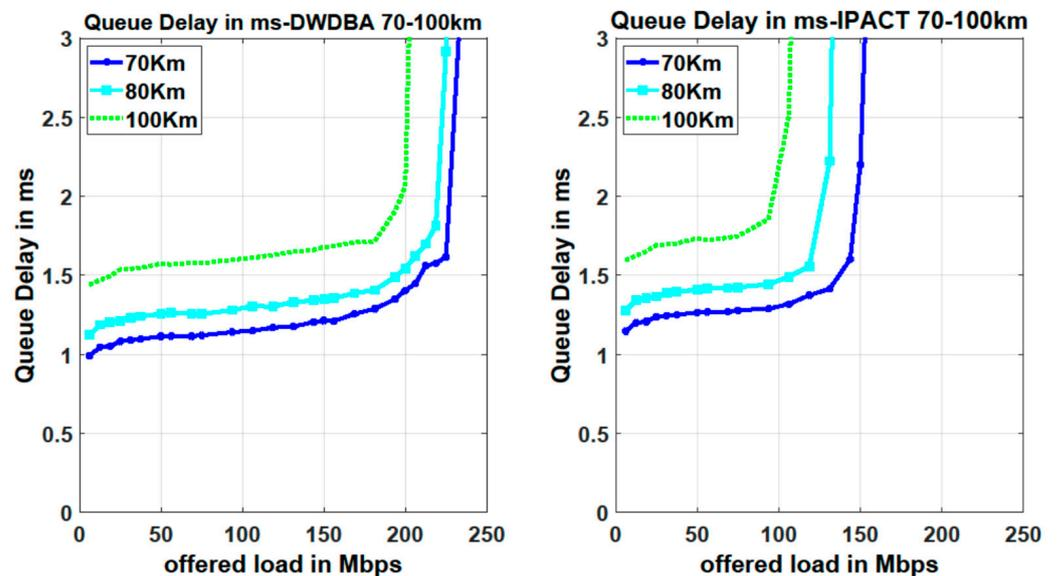
Figure 10. Queue delay for scenario 2 where the ONUs are placed between 70 km and 100 km from OLT for DWDBA (left) and IPACT (right).
