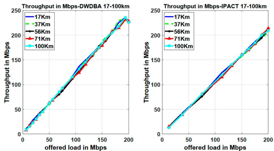
Figure 7. Throughput for scenario 3 where the ONUs are placed between 17 km and 100 km from OLT for DWDBA (left) and IPACT (right).
