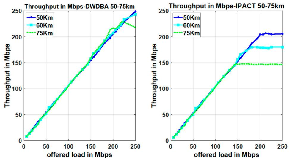
Figure 5. Throughput for scenario 1 where the ONUs are placed between 50 km and 75 km from OLT for DWDBA (left) and IPACT (right).
