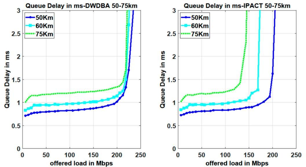
Figure 9. Queue delay for scenario 1 where the ONUs are placed between 50 km and 75 km from OLT for DWDBA (left) and IPACT (right).
