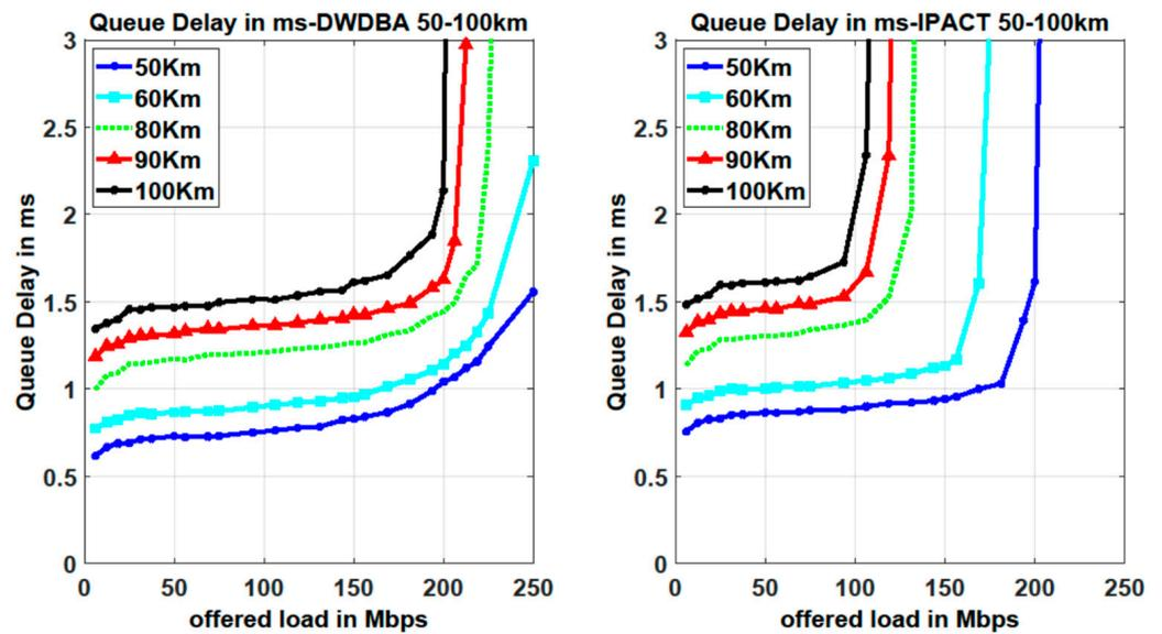
Figure 12. Queue delay for ONUs placed between 50 km and 100 km from OLT for DWDBA (left) and IPACT (right).
