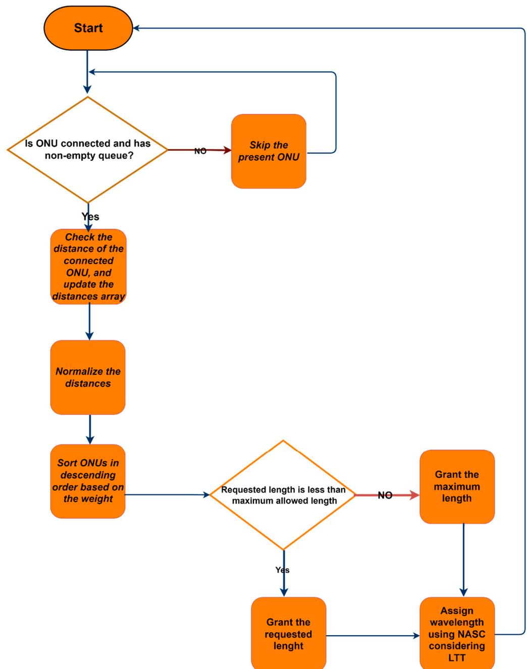
**Figure 3.** Flowchart of the DWDBA algorithm.
