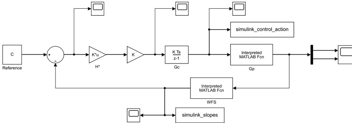
**Figure 3.** Block diagram of OOMAO simulation integrated with Simulink.  $G_c$  indicates the controller (in the example, a discrete-time Integral controller),  $G_p$  is the atmospheric turbulence process,  $H^*$  indicates the reconstruction matrix, and WFS the model of the Shack-Hartman wavefront sensor.
