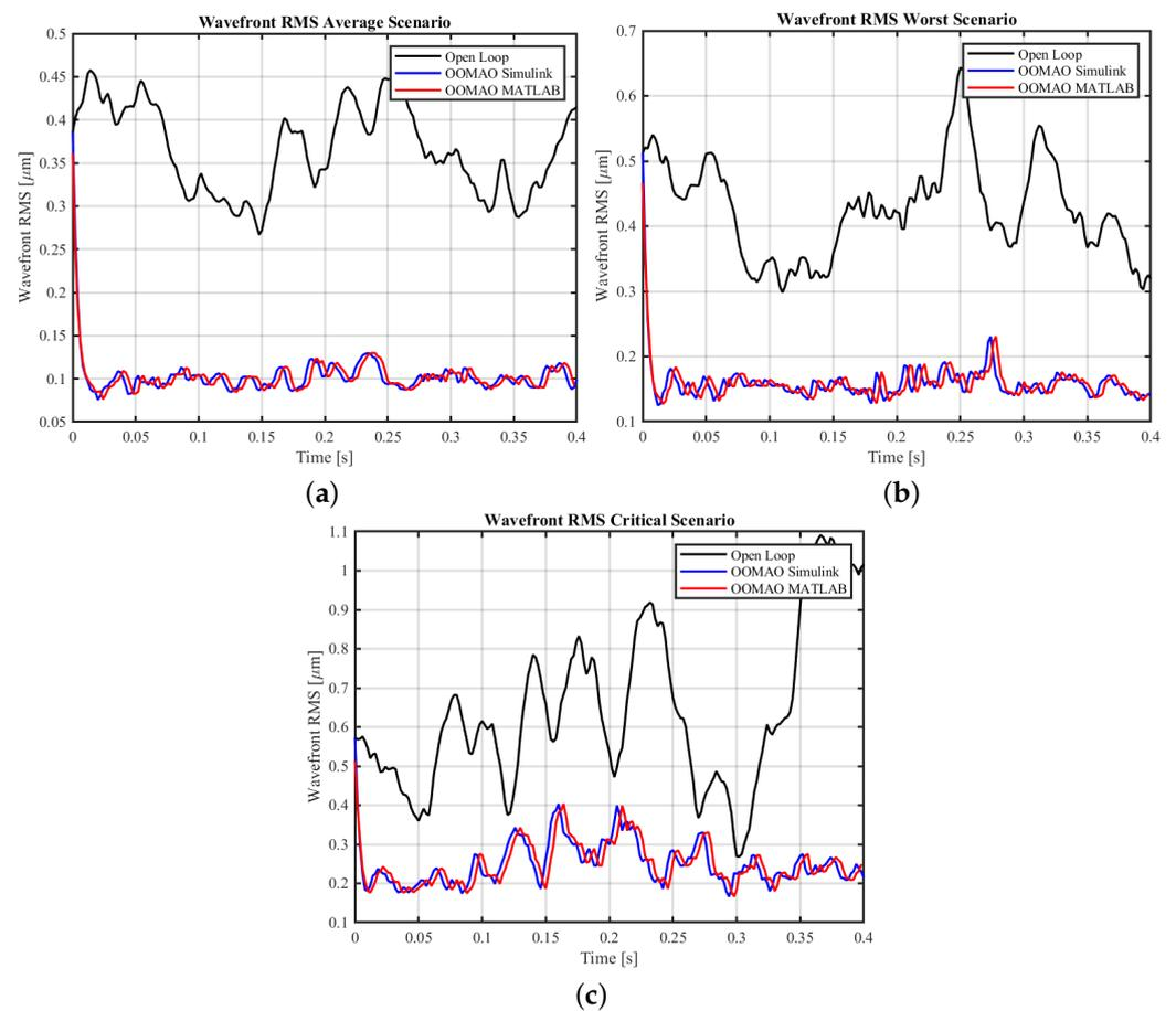
**Figure 5.** Wavefront RMS values over time for an open loop (black line), with the controller implemented in Simulink using the adaptation layer (blue line), and with the controller directly implemented in MATLAB without the adaptation layer (red line). Simulation scenarios: (a) typical case, (b) worst case, and (c) critical case. The delay between the curves of “OOMAO Simulink” and “OOMAO MATLAB” occurs due to internal processing aspects of the Simulink, not affecting the calculation.
