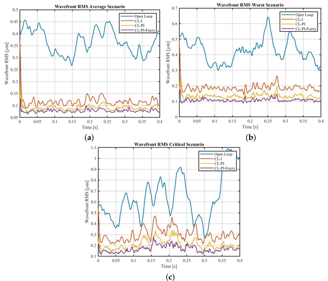
**Figure 12.** Wavefront RMS values over time for all the control strategies implemented: open loop, in a closed loop with I (CL-I), PI (CL-PI), and fuzzy PI (CL-PI-Fuzzy) controllers. Simulation scenarios: (a) typical case, (b) worst case, and (c) critical case.
