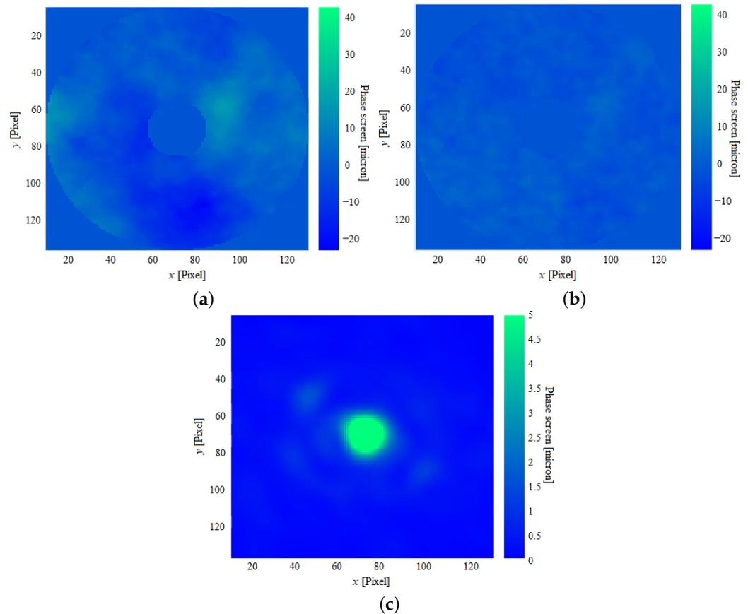
**Figure 4.** The total incident wavefront is represented in (a). The residual wavefront and the accumulated wavefront after the Integral controller action are indicated, respectively, in (b,c). The axes  $x$  and  $y$  represent the camera with  $128 \times 128$  pixels and the  $z$  axis is the phase [ $\mu\text{m}$ ].
