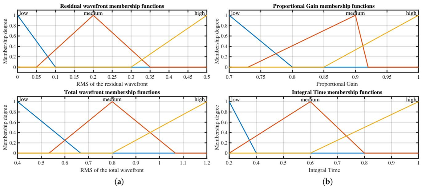
**Figure 9.** Triangular membership functions with the linguistic terms low, medium, and high for: (a) input variables (RMS value of the residual and total wavefront error), and (b) output variables (proportional gain and integral time).
