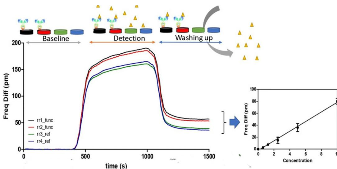
**Figure 3.** Biosensor sensogram detection of *E. coli* O157:H7 or its verotoxins. A schematic sensogram obtained by the immunosensor setup reader against the target antigen is included. Here are represented the resonance obtained versus the test time. The hardware and software components of the setup reader translate the optical signals obtained in the detection sensogram into measurable resonance values: freq. diff (pm) against the concentration of the target antigen (log CFU/mL).
