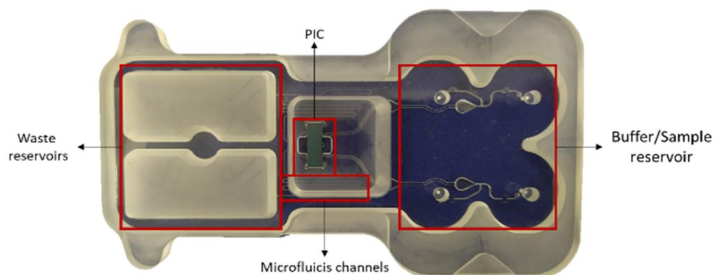
**Figure 2.** PIC ensembled into microfluidic cartridge.
