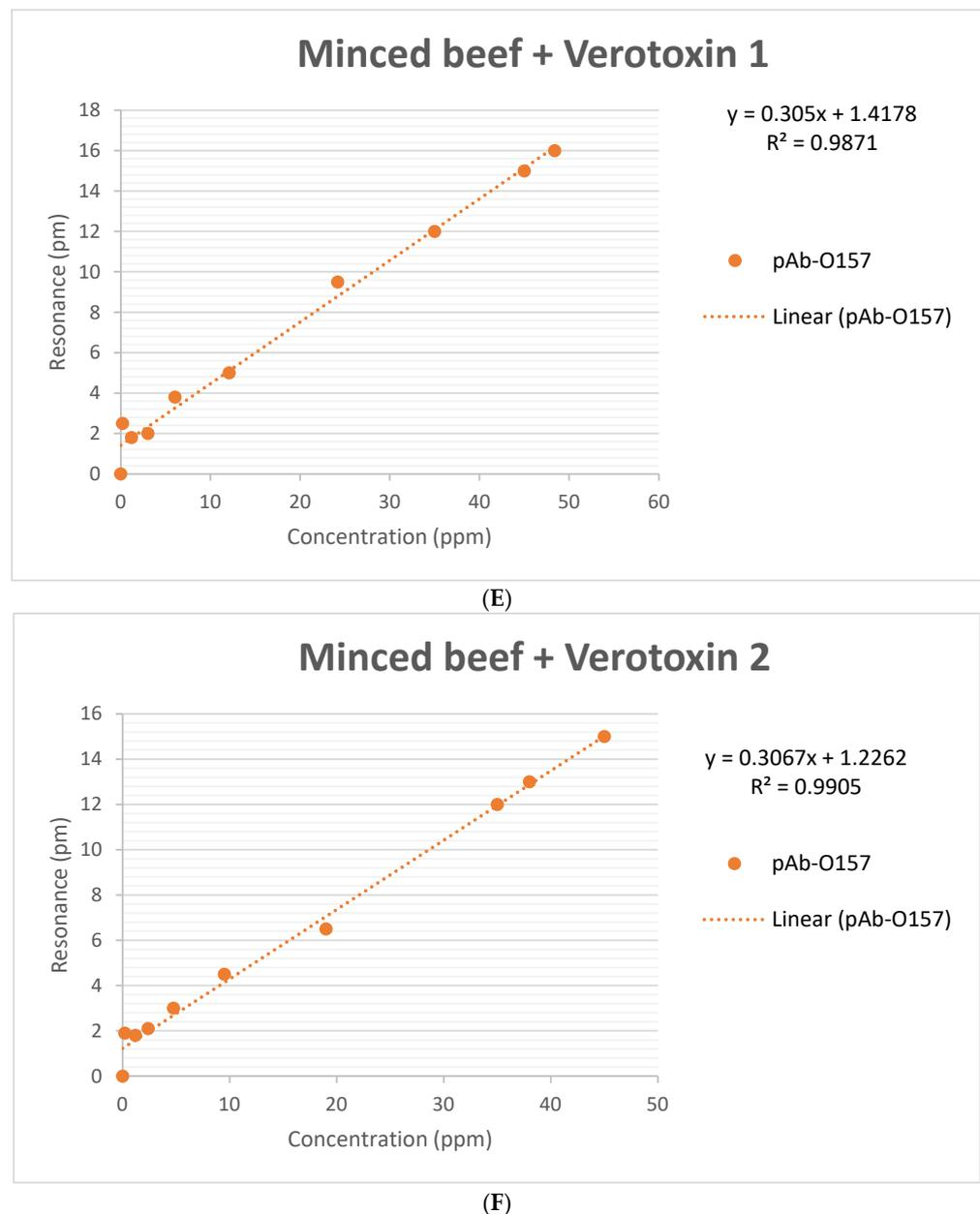
**Figure 6.** Validation calibration curves against antigens of *E. coli* O157:H7. (A) Biosensor calibration curve against *E. coli* O157:H7. (B) Biosensor calibration curve against verotoxin 1 (VTx1). (C) Biosensor calibration curve against verotoxin 2 (VTx2) (D) Biosensor calibration curve against *E. coli* O157:H7-spiked minced beef samples. (E) Biosensor calibration curve against VTx1-spiked minced beef samples. (F) Biosensor calibration curve against VTx2-spiked minced beef samples.
