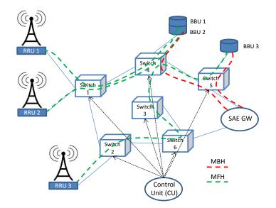
Figure 14. Possible architecture for converged metro-access MBH/MFH network.
