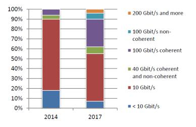
Figure 2. Evolution towards higher capacity channels in the metro network [12].
