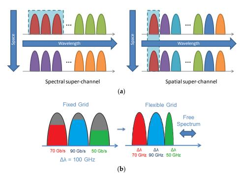
Figure 6. (a) Comparison of spatial and spectral super-channels. (b) Schematic representation of the advantages of flexible grids in terms of spectral efficiency.
