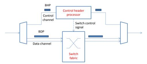
Figure 9. Schematic representation of an OBS router.
