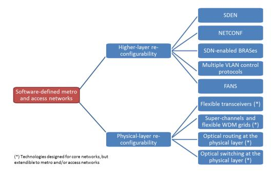
Figure 5. Main solutions for software-defined metro and access networks.
