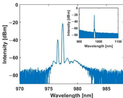
Figure 10. The output spectrum of the double-wavelength fiber oscillator with 160-mW output power.
