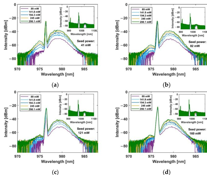
**Figure 3.** Four figures of output spectra via pump power corresponding to four seed power values corresponding to 41 mW, 82 mW, 121 mW, 160 mW (a–d).
