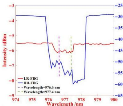
Figure 9. The transmission spectra of HR-FBG and LR-FBG.
