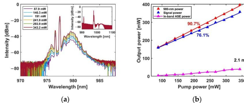
**Figure 12.** (a) The variation of output spectra with pump power. (b) The variation of output power with pump power by using the double-wavelength seed source.
