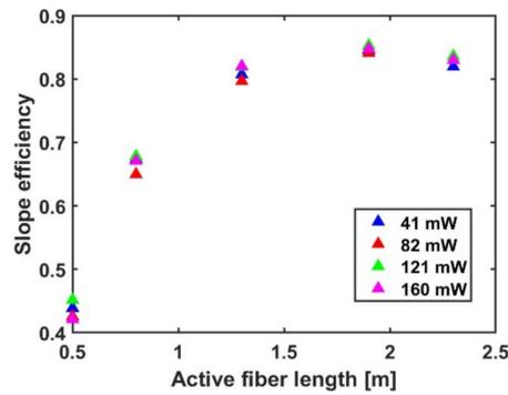
Figure 5. The slope efficiency of output emission around 980 nm via active fiber length.
