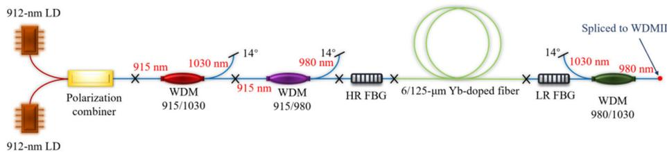
Figure 8. The experimental setup of the double-wavelength fiber oscillator.
