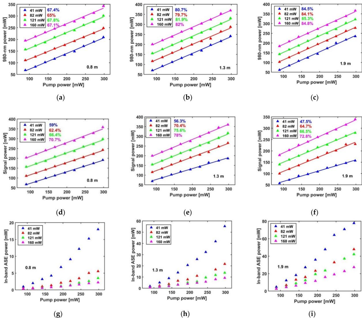
Figure 6. Output power of (a–c) emission around 980 nm and (d–f) signal light and (g–i) in-band ASE with 0.8-m, 1.3-m, and 1.9-m active fibers, respectively.
