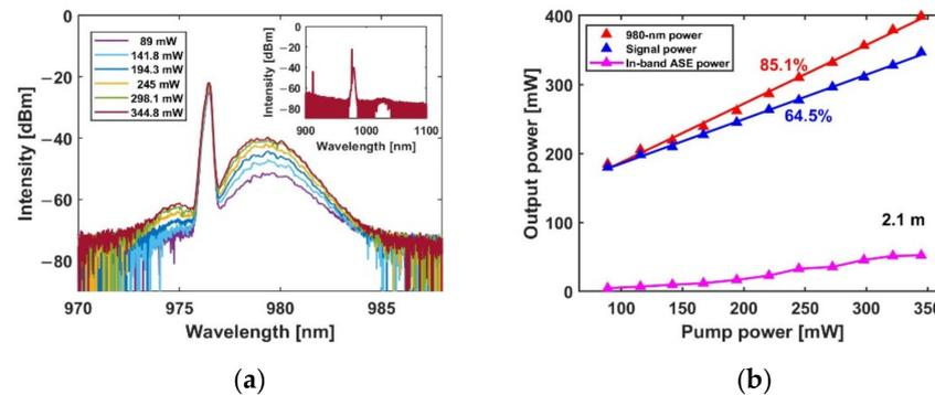
**Figure 11.** (a) The variation of output spectrum with pump power; (b) the variations of output power with pump power by using the 976.5-nm LD seed source.
