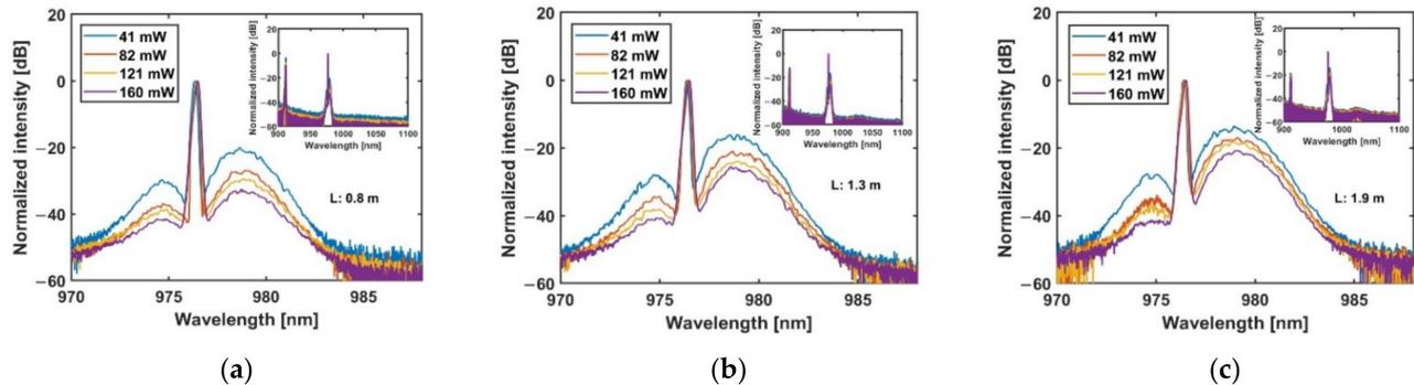
**Figure 7.** The variations of output spectrum with various seed power corresponding to 0.8-m, 1.3-m, and 1.9-m active fibers (a–c).
