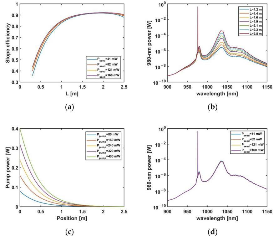
**Figure 1.** (a) The variations of slope efficiency with active fiber length. (b) The variation of output spectrum with active fiber length. The pump and seed power are 400 mW and 160 mW, respectively. (c) The variations of pump power along the active fiber. (d) The variation of spectrum with seed power. The active fiber length and pump power are 2.0 m and 160 mW, respectively.
