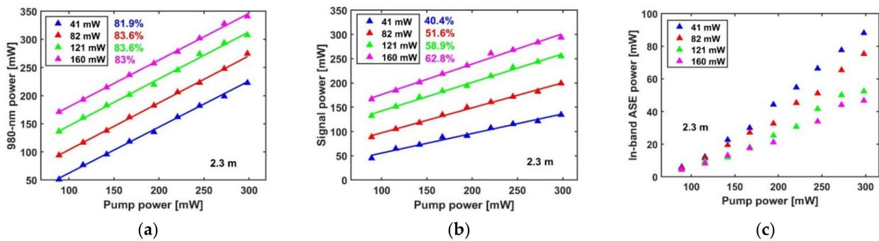
**Figure 4.** Output power of (a) emission around 980 nm and (b) signal light and (c) in-band ASE with 2.3-m active fiber.
