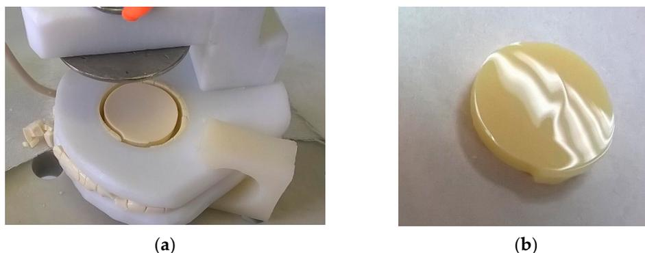
**Figure 9.** Dry compact obtained by vertical EPD from YLO\_iA\_1 suspension: (a)–at the beginning of the drying process in the cell; (b) dry compact.
