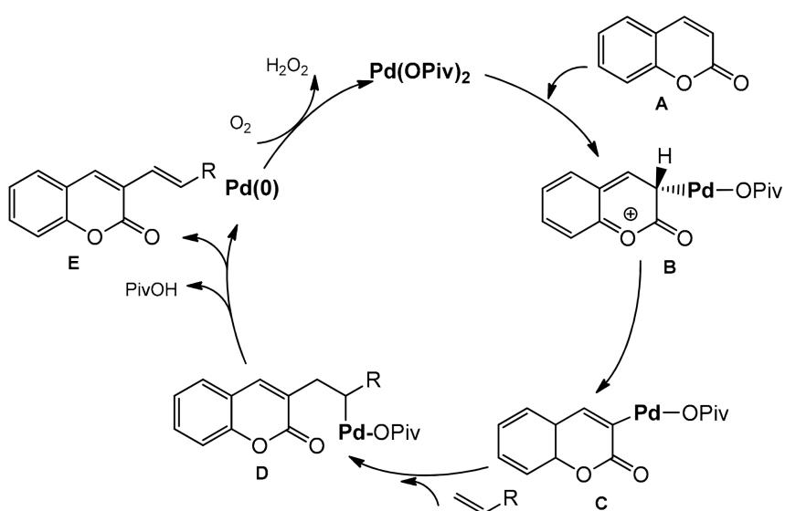
**Scheme 26.** Proposed mechanism of Pd-catalyzed C-3 functionalization.
