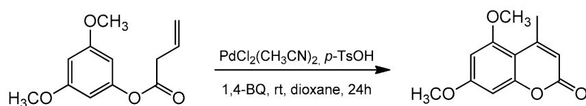
**Scheme 14.** Synthesis of 5,7-dimethoxy-4-methylcoumarin.
