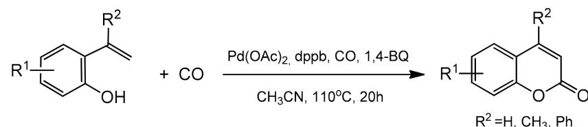
**Scheme 16.** Pd-catalyzed oxidative cyclocarbonylation of 2-vinylphenol.
