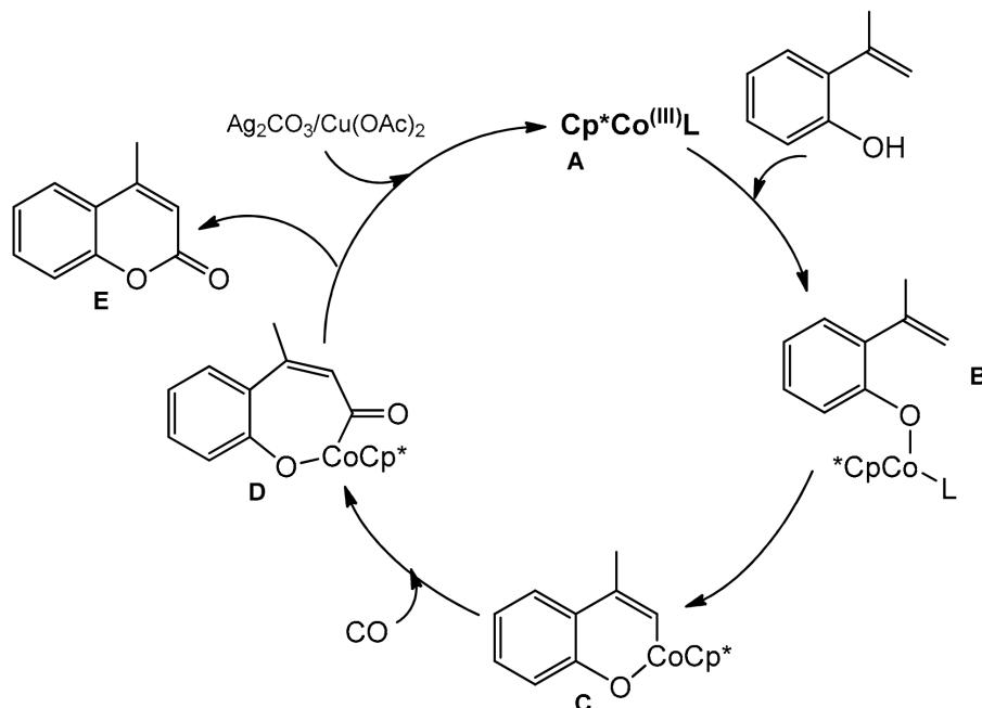
Scheme 18. Mechanism of the Co-catalyzed carbonylation reaction.
