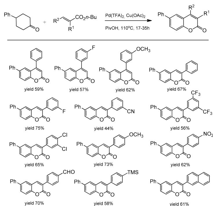
**Scheme 23.** Palladium-catalyzed reaction of 4-phenylcyclohexanone with the alkene substrate.
