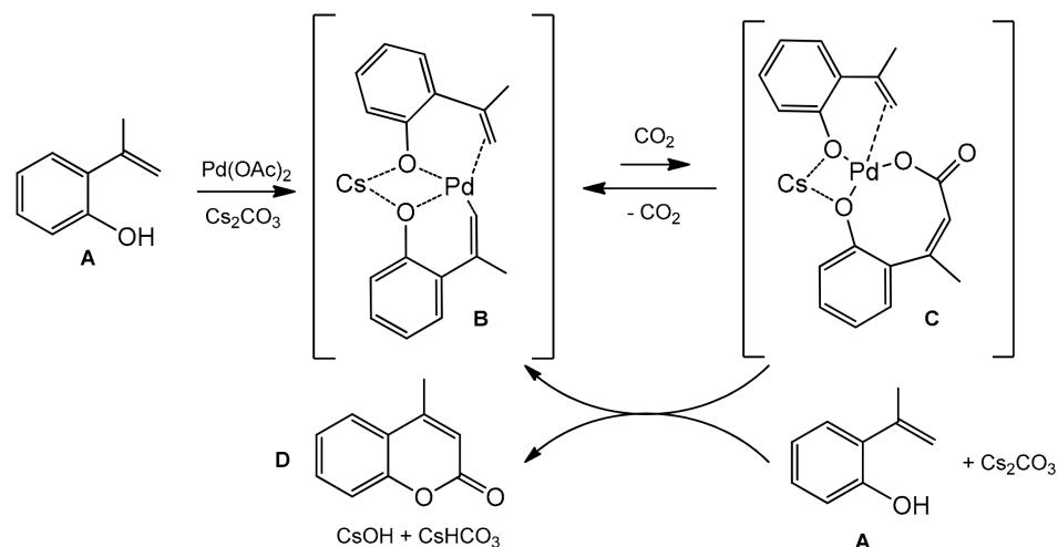
**Scheme 20.** Mechanism of Pd-catalyzed reaction of 2-hydroxystyrenes with carbon dioxide.
