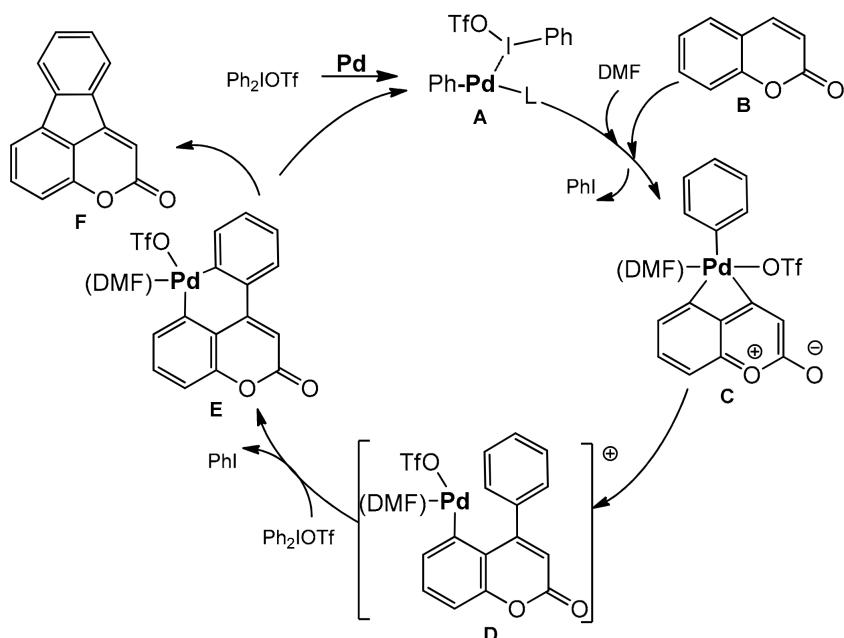
**Scheme 37.** Proposed mechanism of the 4,5 benzocoumarins synthesis.
