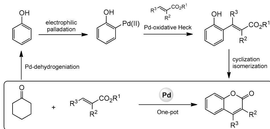
**Scheme 21.** Sequence of reactions for construction of substituted coumarins.
