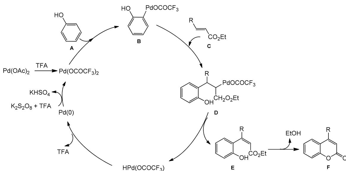
**Scheme 10.** Mechanism of Pd-catalyzed arylation of acrylates.
