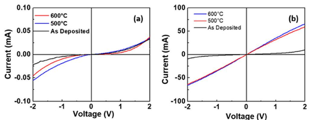
**Figure 11.** I–V curves of (a) Au/Ti/Ga<sub>2</sub>O<sub>3</sub> and (b) Au/Ti/ITO/Ga<sub>2</sub>O<sub>3</sub> contact stacks as a function of annealing temperature. Reproduced from Ref. [100].
