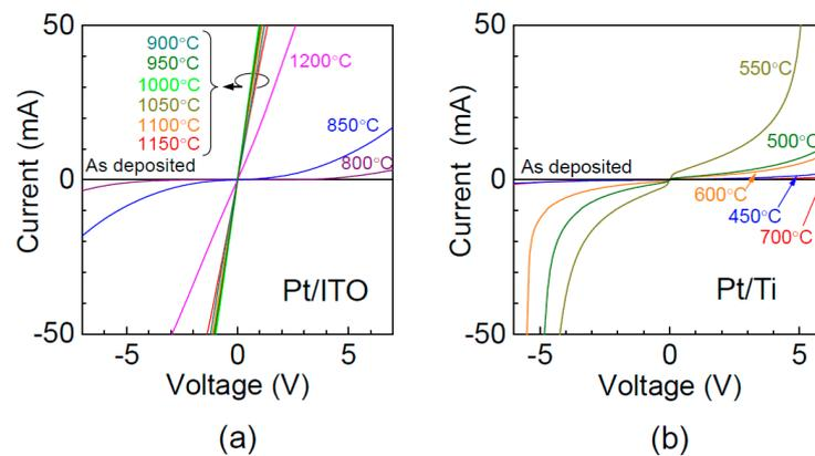
**Figure 10.** Typical I–V characteristics of (a) Pt/ITO and (b) Pt/Ti electrodes annealed at various temperatures. Reproduced from Ref. [99].
