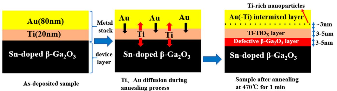
**Figure 2.** Schematic illustrations of Ti/Au metallization layers on Sn-doped  $\beta\text{-Ga}_2\text{O}_3$  with a 1 min 470 °C  $\text{N}_2$  annealing process. Reproduced from Ref. [68].
