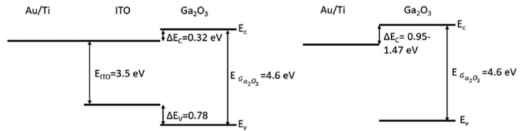
**Figure 12.** Schematics of band offset for Au/Ti/ITO on Ga<sub>2</sub>O<sub>3</sub> and Au/Ti on Ga<sub>2</sub>O<sub>3</sub>. Reproduced from Ref. [100].
