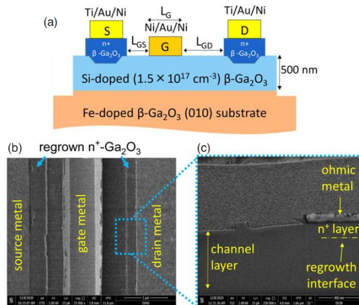
**Figure 9.** (a) Schematic of the fully MOVPE-grown  $\text{Ga}_2\text{O}_3$  MESFET with regrown Ohmic contacts. (b) Top-view SEM image of the MESFET showing the regrown access regions. (c) Cross-sectional SEM image of the contact region showing the estimated regrowth interface. Reproduced from Ref. [36].
