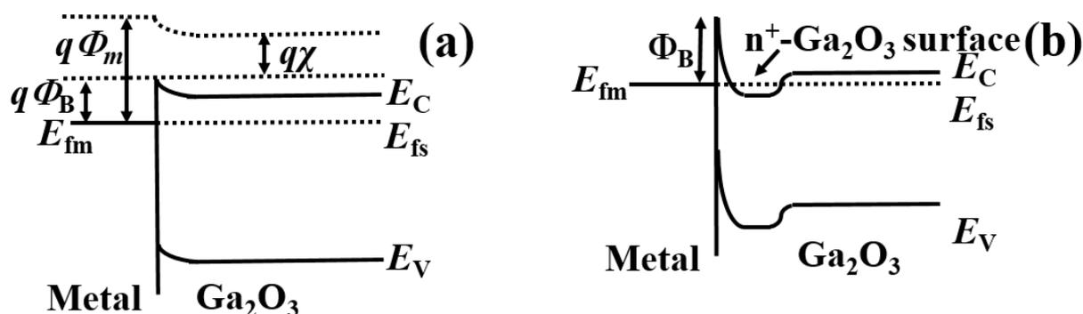
**Figure 1.** Energy-band diagrams of metal–Ga<sub>2</sub>O<sub>3</sub> Schottky contacts with (a) a lower  $\Phi_{bm}$  and (b) an n<sup>+</sup>-doped Ga<sub>2</sub>O<sub>3</sub> region.
