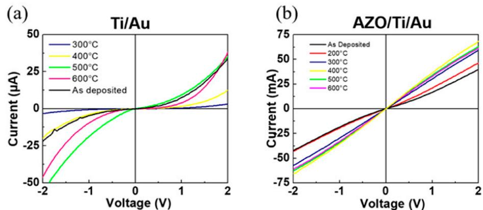
**Figure 13.** I–V curves of (a) Au/Ti/Ga<sub>2</sub>O<sub>3</sub> and (b) Au/Ti/AZO/Ga<sub>2</sub>O<sub>3</sub> contact stacks as a function of annealing temperature from as-deposited samples (black lines) to 600 °C (purple lines). The 200 °C data were similar to those of the as-deposited samples, and the contact resistance decreased with temperature in the AZO-based contacts. Reproduced from Ref. [101].
