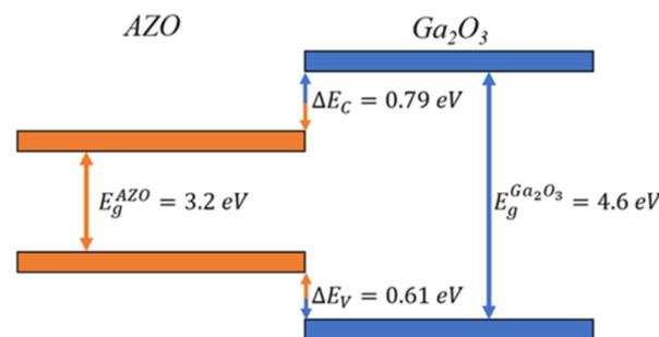
**Figure 14.** Schematic of band offset for AZO on Ga<sub>2</sub>O<sub>3</sub>. Reproduced from Ref. [101].
