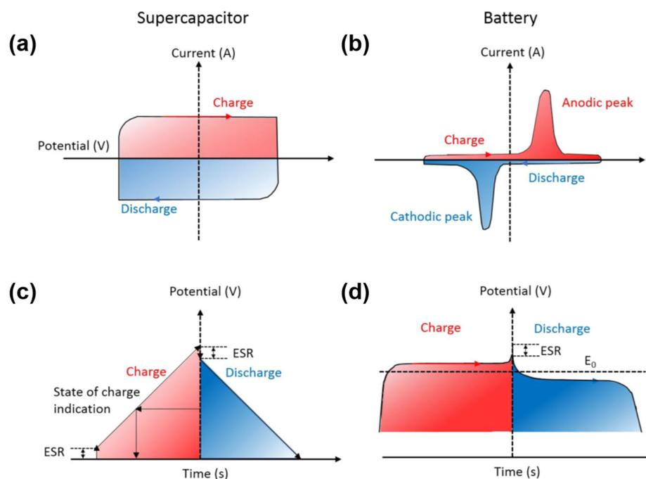
**Figure 4.** (a,b) Cyclic voltammetry (CV) curves and (c,d) galvanostatic charge-discharge (GCD) curves of supercapacitors and batteries. Reproduced with permission from [26]. Copyright 2018 American Chemical Society.
