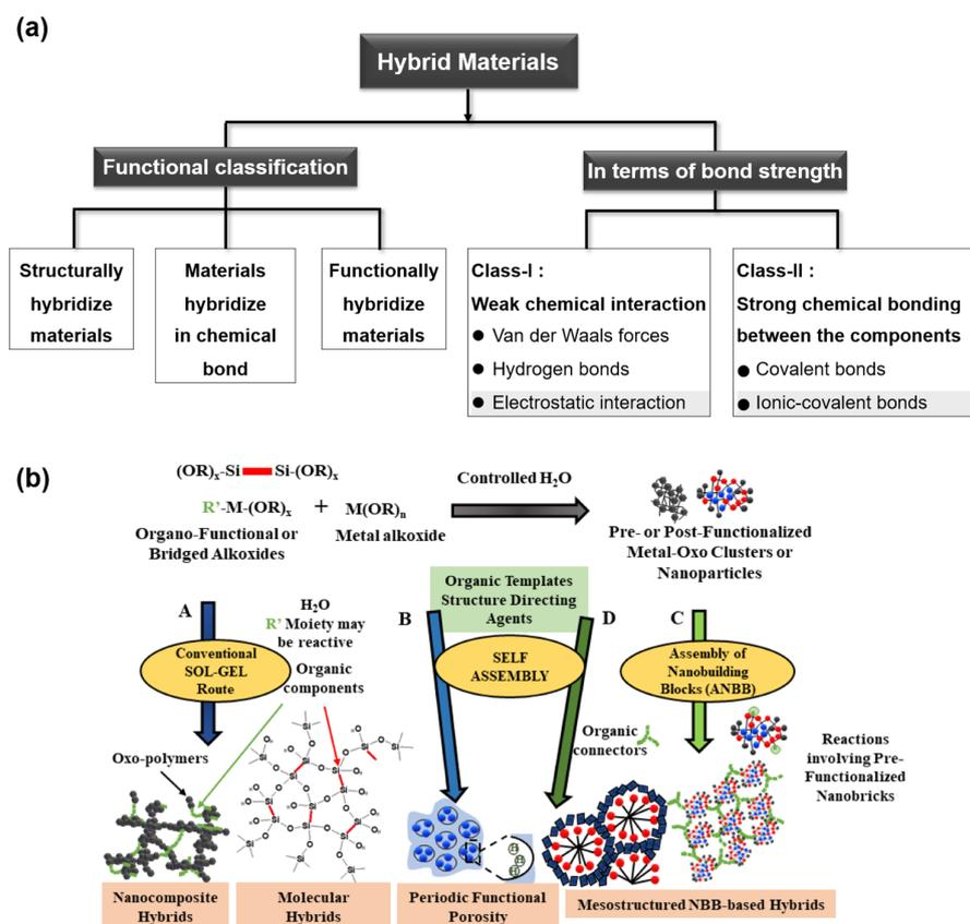
**Figure 5.** (a) The general classification of hybrid materials and (b) several general approaches for the design of hybrid nanostructured materials prepared by various routes (A: homogenous molecular organic-inorganic materials, B: self-assembling procedures into account, C: assembling of well-defined nanobuilding blocks and D: combination of self-assembly and nanobuilding block approaches). (b) is reprinted/adapted with permission from Ref. [34] 2021, MDPI.
