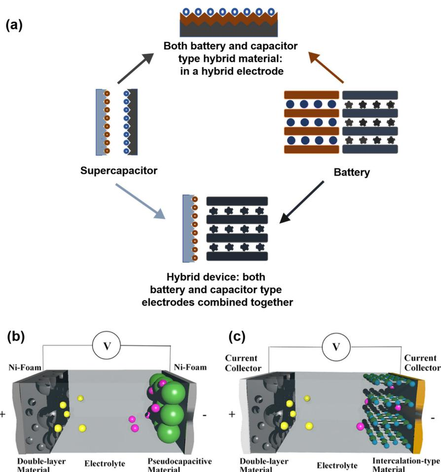
**Figure 6.** (a) Schematic representation of the development of a hybrid energy storage system through the combination of hybrid materials as electrodes for both supercapacitors and batteries. Different types of hybrid energy storage devices (b) asymmetric supercapacitors. (c) Battery supercapacitors. (b,c) are reproduced with permission from [150]. Copyright 2019 Elsevier.
