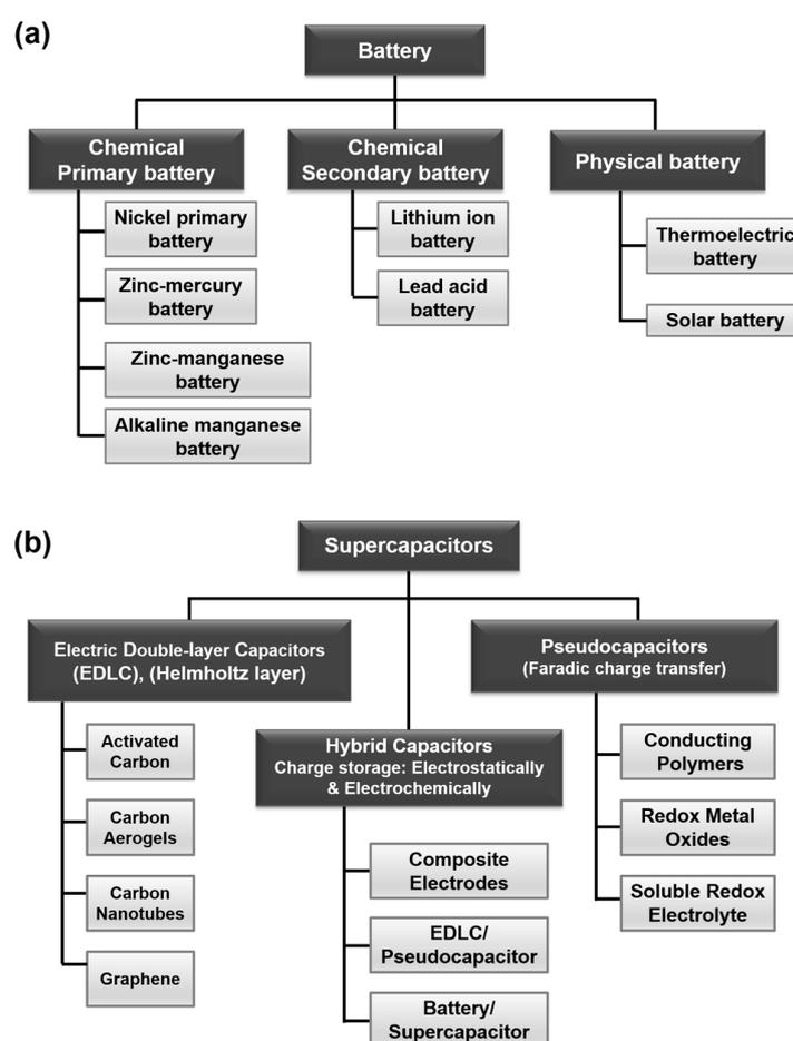
**Figure 3.** Classifications of: (a) batteries; and (b) supercapacitors based on electrode materials and charge storage mechanism.
