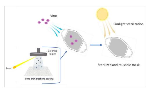
**Figure 4.** The mask, made using an ultra-thin graphene layer deposited by the Laser dual method, is reusable and sterilizable with the aid of solar radiation.
