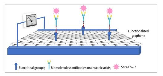
Figure 2. Biosensor with functionalized graphene containing biomolecules attracting SARS-CoV-2.
