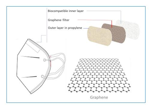
Figure 3. Mask with graphene filter.
