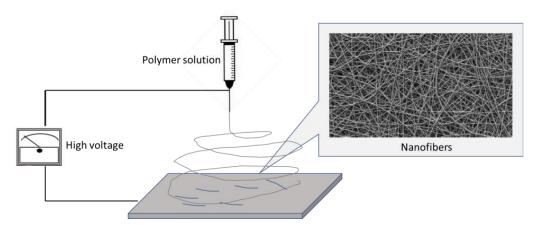
Figure 8. Electrospinning nanofibers at high voltage.
