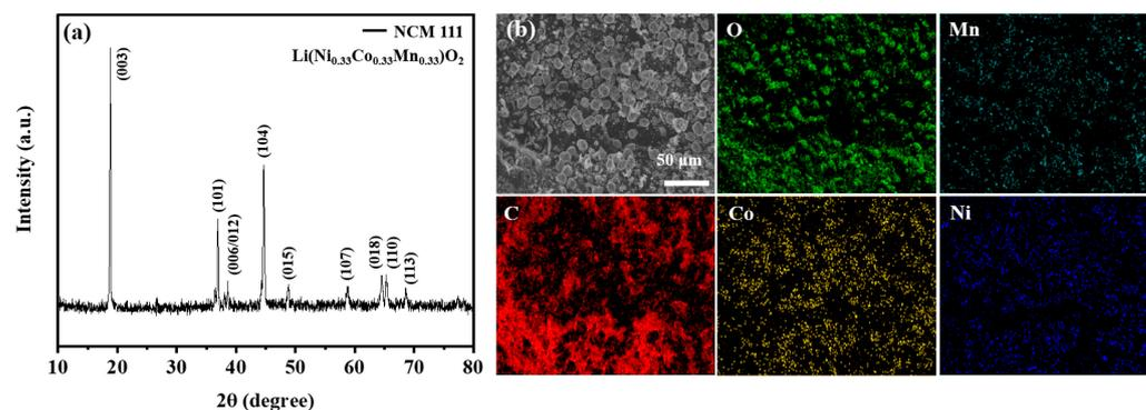
**Figure 1.** (a) XRD data of the black powder obtained from cathode of the end-of-life lithium-ion battery. (b) Micrographs of black powder and corresponding EDS mappings of different elements.
