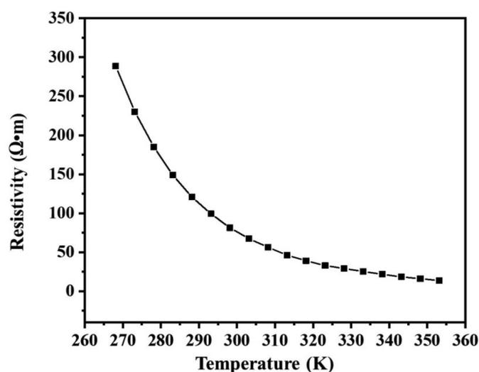
**Figure 6.** Resistivity of the sintered Ni-Co-Mn oxides in the temperature range between 268 K and 353 K.
