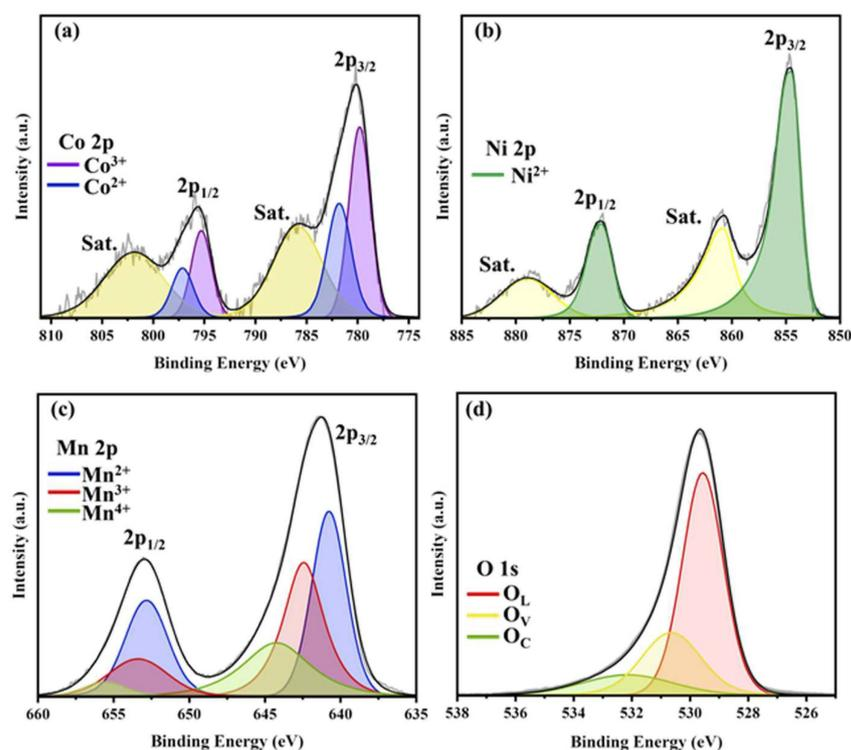
**Figure 5.** XPS analysis data of (a) Co 2p, (b) Ni 2p, (c) Mn 2p, and (d) O 1s of the sintered Ni-Co-Mn oxides.
