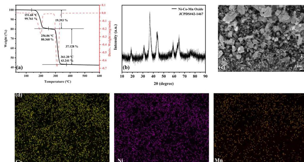
**Figure 3.** (a) TGA-DTG data, (b) XRD data, (c) micrograph, and (d) corresponding EDS mappings of the different elements of the oxide powder.
