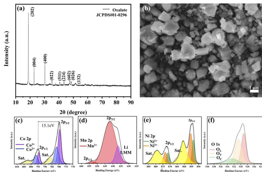
**Figure 2.** (a) XRD patterns and (b) micrographs of the Ni-Co-Mn oxalate powder after leaching process followed by chemical synthesis, as well as XPS analysis data of (c) Co 2p, (d) Mn 2p, (e) Ni 2p, and (f) O 1s.
