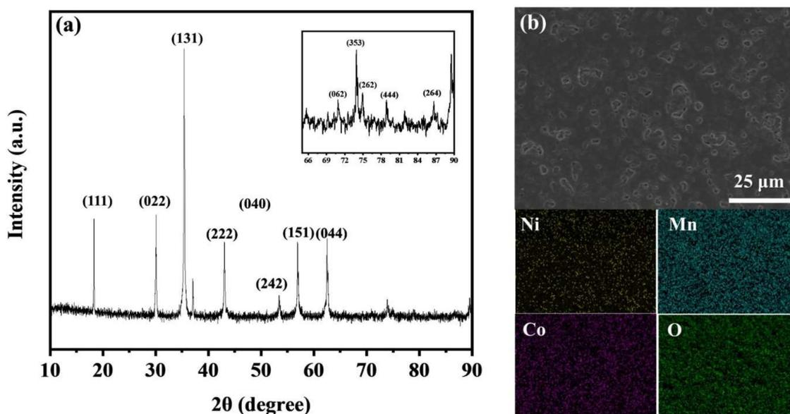
**Figure 4.** (a) XRD data and (b) micrographs and corresponding EDS mapping of sintered Ni-Co-Mn oxides.
