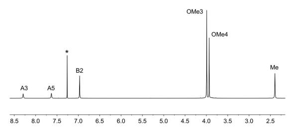
**Figure 1.** The 500 MHz <sup>1</sup>H NMR spectrum of  $[Cu(4)_2][PF_6]$  (CDCl<sub>3</sub>). \* = residual CHCl<sub>3</sub>. Chemical shifts in  $\delta$ /ppm. See Scheme 1 for labelling.
