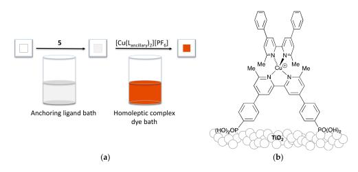
**Figure 4.** (a) The SALSAC approach to functionalization of a glass  $FTO/TiO_2$  electrode surface with a heteroleptic  $[Cu(L_{anchor})(L_{ancillary})]^+$  dye. Transparent electrodes were used for absorption spectroscopy, and  $TiO_2$  with a scattering layer was used for DSSC measurements. (b) Surface-anchored  $[Cu(5)(1)]^+$ .
