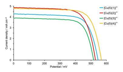
Figure 7. J–V curves for the best performing DSSCs containing dyes  $[Cu(5)(L_{ancillary})]^+$   $(L_{ancillary} = 1-4)$ .
