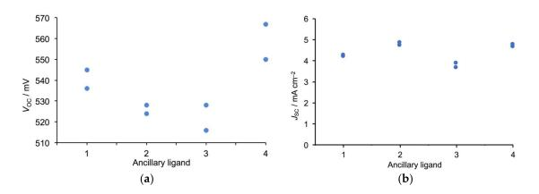
**Figure 8.** Trends in values of (a)  $V_{OC}$  and (b)  $J_{SC}$  for duplicate DSSCs containing the dyes  $[Cu(5)(1)]^+$  (Ph groups),  $[Cu(5)(2)]^+$  (4-MeOC<sub>6</sub>H<sub>4</sub> groups),  $[Cu(5)(3)]^+$  (3,5-(MeO)<sub>2</sub>C<sub>6</sub>H<sub>3</sub> groups), or  $[Cu(5)(4)]^+$  (3,4,5-(MeO)<sub>3</sub>C<sub>6</sub>H<sub>2</sub> groups).
