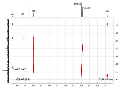
**Figure 2.** Part of the HMBC spectrum (500 HMz  $^{1}$ H, 126 MHz  $^{13}$ C) of [Cu(4)<sub>2</sub>][PF<sub>6</sub>] (CDCl<sub>3</sub>). \* = residual CHCl<sub>3</sub>.
