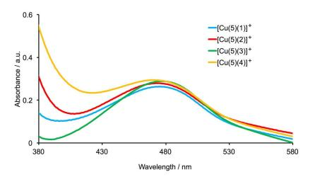
**Figure 5.** Solid-state absorption spectra of FTO/TiO<sub>2</sub> electrodes functionalized with  $[Cu(5)(L_{ancillary})]^+$  dyes ( $L_{ancillary} = 1, 2, 3, \text{ or } 4$ ).
