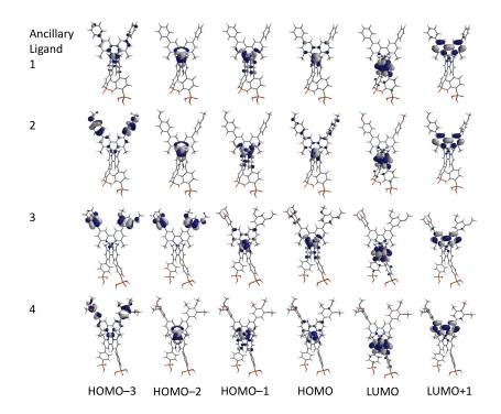
**Figure 10.** Characteristics of the MOs from HOMO-3 to LUMO+1 of  $[Cu(5)(1)]^+$  (top row),  $[Cu(5)(2)]^+$ ,  $[Cu(5)(3)]^+$ , and  $[Cu(5)(4)]^+$  (bottom row). The orientation of the complex is the same in each figure, with anchor 5 as the lower ligand. (DFT B3LYP level with a 6-31G\* basis set in vacuum.).
