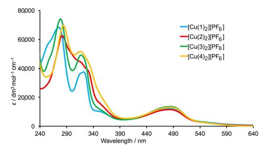
**Figure 3.** Solution absorption spectra of the homoleptic copper(I) complexes (CH<sub>2</sub>Cl<sub>2</sub>,  $1 \times 10^{-5}$  mol dm<sup>-3</sup>).
