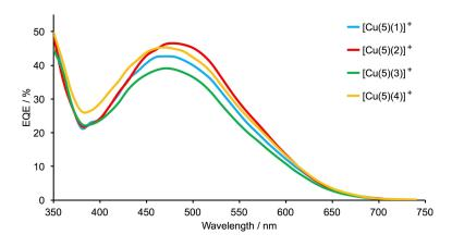
Figure 9. EQE spectra for the best performing DSSCs containing dyes  $[Cu(5)(L_{ancillary})]^+$   $(L_{ancillary} = 1-4)$ .
