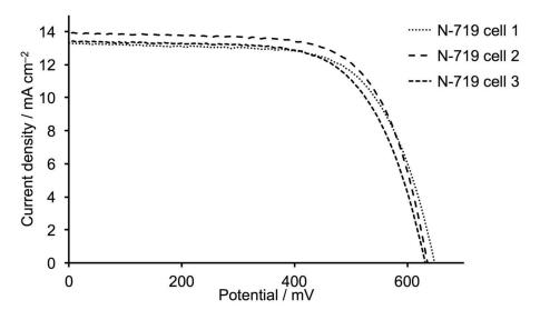
**Figure 6.** *J–V* curves for three N719 reference cells (DSSCs were fully masked).
