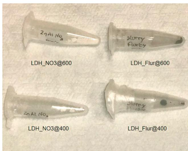
**Figure S4.** Picture of the samples after calcination showing that the inorganic calcined LDHs remain white, while organic intercalated LDHs are black after the calcination.
