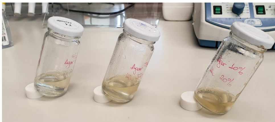
Figure S2. Agar solutions (from left to right: 2.5, 5.0 and 10.0% w/v ) in HAc 20% v/v .
