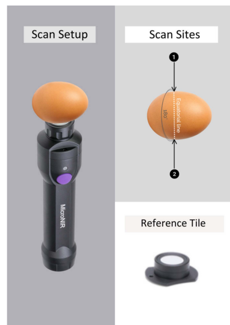
Figure 1. Set up, scan sites and reference tile (Spectralon®) used to collect the NIR spectra of the egg samples.
