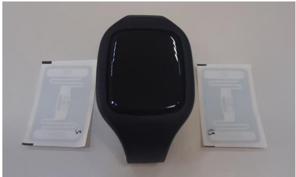
Figure 6. Wearable RFID reader and RFID tags.
