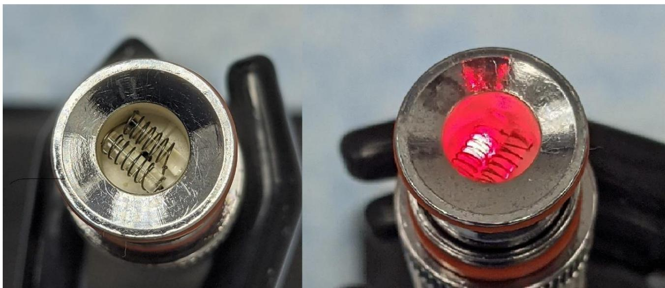
**Figure 2.** Kind Dream heating element (left—coils, right—heated coils).
