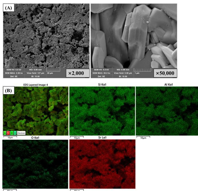
Figure 5. (A) SEM images and (B) EDS mapping of solidified product.
