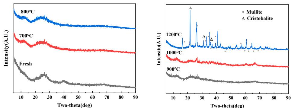
**Figure 2.** XRD patterns of allophanes sintered at different temperatures.
