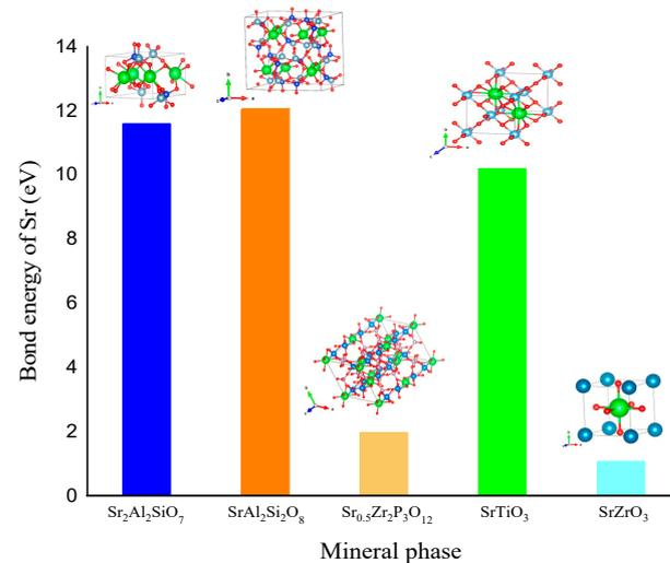
Figure 14. Bond energies of Sr in different mineral phases.
