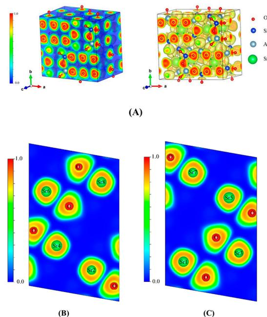
**Figure 12.** (A) Three-dimensional ELF diagrams of  $\text{SrAl}_2\text{Si}_2\text{O}_8$  (B,C) are two-dimensional electron localization diagrams of  $\text{SrAl}_2\text{Si}_2\text{O}_8$  on the cross-section at 3.24 and 9.72 Å from the set (0 1 0) crystal plane, respectively.
