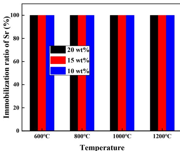
**Figure 3.** Sr immobilization ratios at different sintering temperatures.
