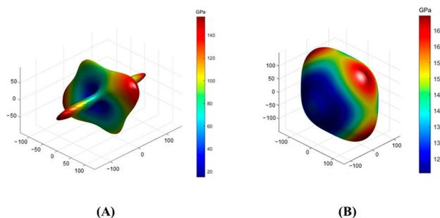
Figure 8. Anisotropy of the Young’s modulus in (A)  $\text{SrAl}_2\text{Si}_2\text{O}_8$  and (B)  $\text{Sr}_2\text{Al}_2\text{SiO}_7$ .
