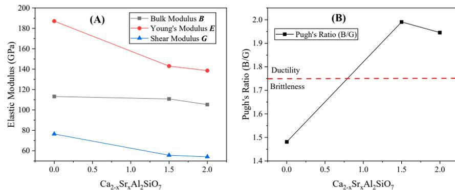
**Figure 11.** (A) Elastic modulus and (B) Pugh's ratio of  $\text{Ca}_{2-x}\text{Sr}_x\text{Al}_2\text{SiO}_7$ .
