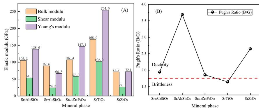
Figure 15. (A) Elastic modulus and (B) Pugh's ratios of different mineral phases.
