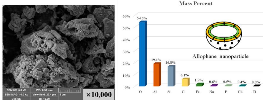
**Figure 1.** SEM images (left) and principal compositions of natural allophanes (right).
