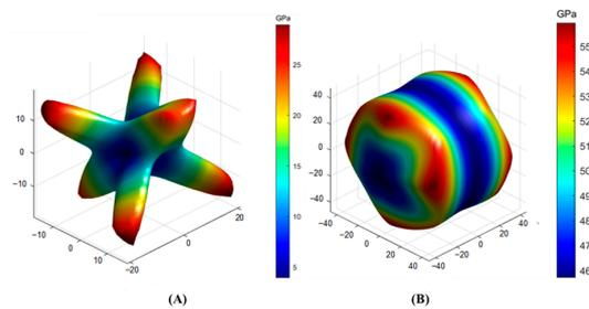
**Figure 9.** Anisotropy of the shear modulus in (A)  $\text{SrAl}_2\text{Si}_2\text{O}_8$  and (B)  $\text{Sr}_2\text{Al}_2\text{SiO}_7$ .
