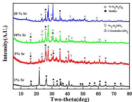
Figure 4. XRD patterns of solidified products at 1200 °C.
