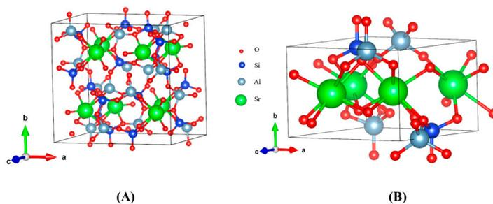
**Figure 6.** Structures of (A) SrAl<sub>2</sub>Si<sub>2</sub>O<sub>8</sub> and (B) Sr<sub>2</sub>Al<sub>2</sub>SiO<sub>7</sub> after optimization.
