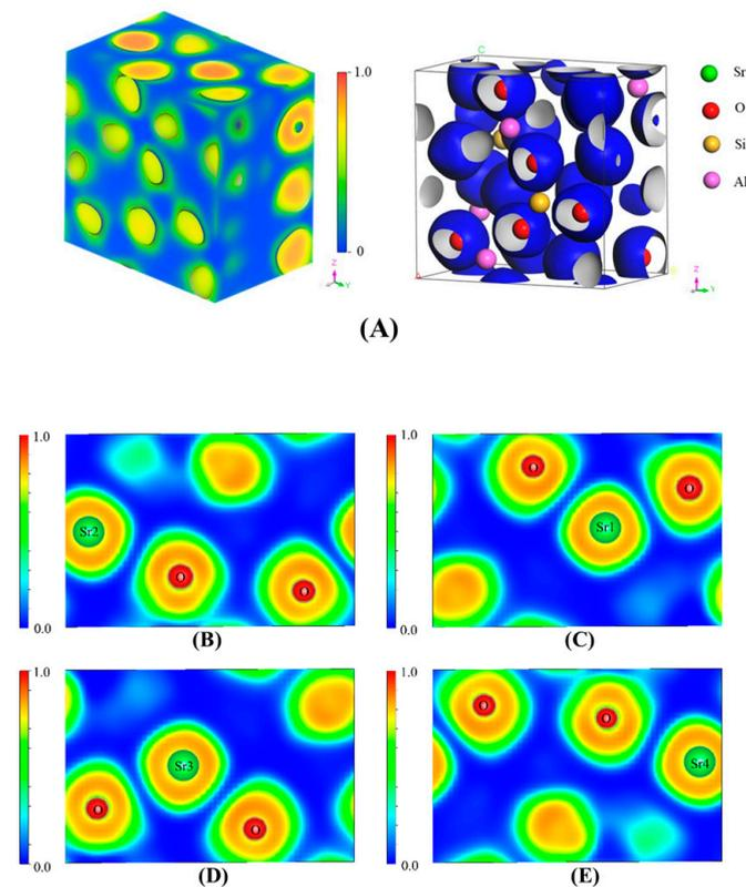
**Figure 13.** (A) Three-dimensional ELF diagrams of  $\text{Sr}_2\text{Al}_2\text{SiO}_7$  (B–E) are two-dimensional electron localization diagrams of  $\text{Sr}_2\text{Al}_2\text{SiO}_7$  on the cross-section at 1.175, 2.74, 5.09, and 6.66 Å from the set (1 0 0) crystal plane, respectively.
