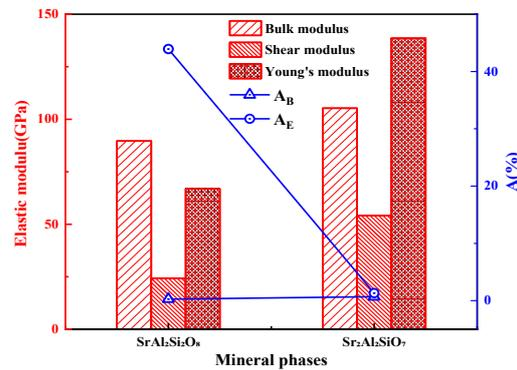
Figure 7. Elastic modulus and the anisotropy of  $\text{SrAl}_2\text{Si}_2\text{O}_8$  and  $\text{Sr}_2\text{Al}_2\text{SiO}_7$ .
