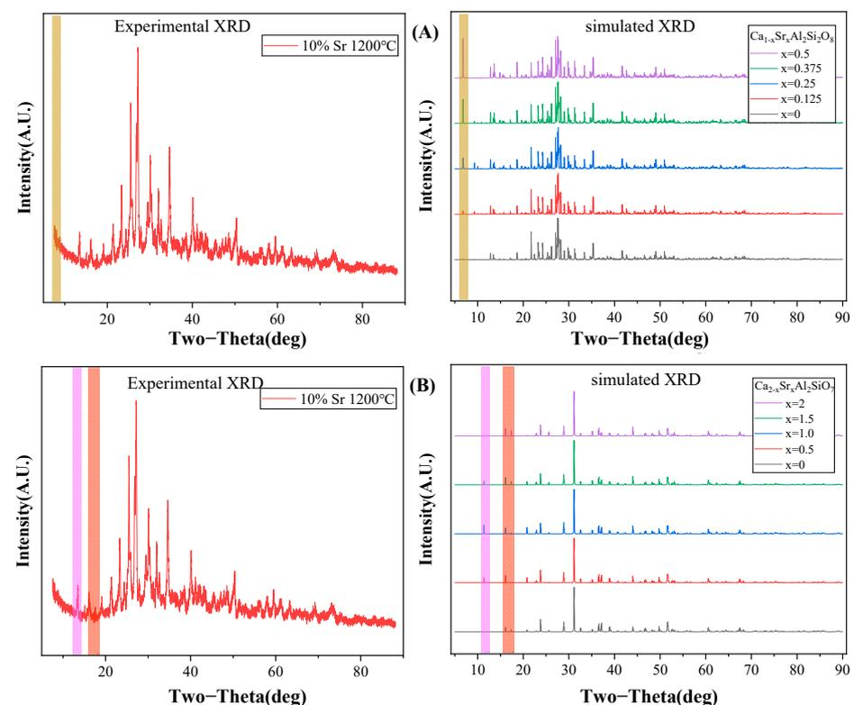
**Figure 10.** Comparison of experimental and simulated XRD patterns: (A)  $\text{SrAl}_2\text{Si}_2\text{O}_8$  and  $\text{Ca}_{1-x}\text{Sr}_x\text{Al}_2\text{Si}_2\text{O}_8$ , and (B)  $\text{Sr}_2\text{Al}_2\text{SiO}_7$  and  $\text{Ca}_{2-x}\text{Sr}_x\text{Al}_2\text{SiO}_7$ . (Green column:  $2\theta = 6.8^\circ$ ; pink column:  $2\theta = 11.38^\circ$ ; red column:  $2\theta = 16.12^\circ$  and  $17.38^\circ$ ).
