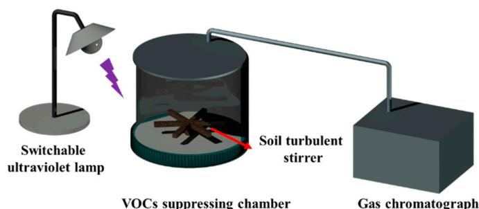
**Figure 1.** System for evaluating the VOC-suppressing foam.
