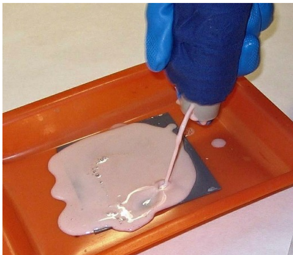
Figure 4. Decontamination of surfaces by the Hvezda two-chamber foam applicator.
