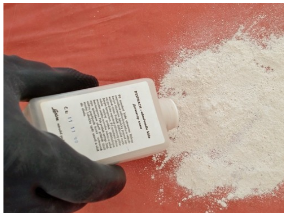
Figure 1. Application of Desprach sorbent to a contaminated surface.
