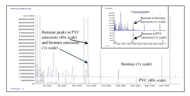
**Figure 1.** Overlaid GC-MS chromatograms of emissions from burning biomass compared to burning PVC pipes. Note that the scale for PVC emissions is expanded forty-fold to show the presence of about 85 volatile organic compounds (VOCs) detected at trace levels. The inset figure shows the same chromatograms on a common scale and the presence of about six major components in the burning PVC emissions.
