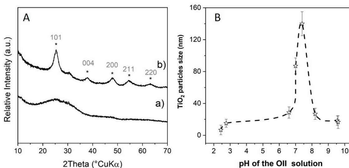
**Figure 1.** (A) PXRD of (a) colloidal TiO<sub>2</sub> freshly prepared, (b) colloidal TiO<sub>2</sub> after three months of storage at 4 °C. (B) Evolution of the TiO<sub>2</sub> particle size during titration with concentrated KOH.
