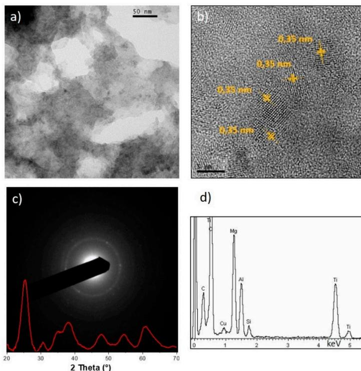
**Figure 5.** TEM and HRTEM analysis of the [MgAl/TiO<sub>2</sub>]<sub>2</sub> nanocomposite obtained by coprecipitation (a) TEM image, (b) HRTEM image, (c) SAED pattern, and (d) EDX spectrum from TEM.
