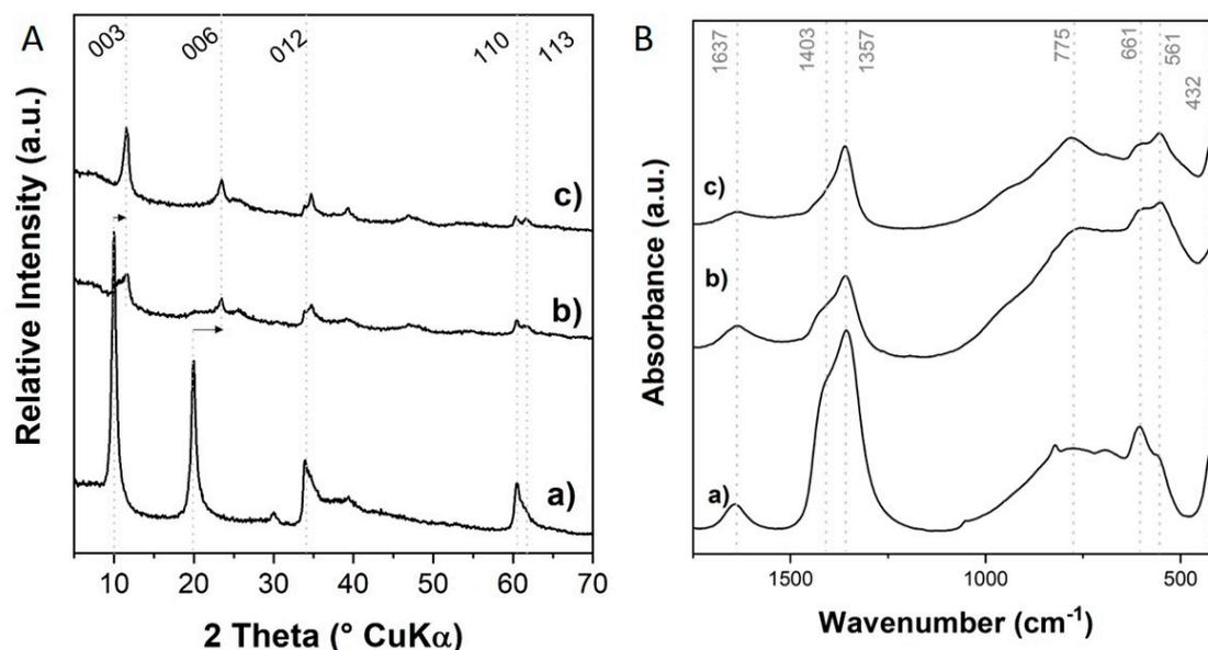
**Figure 2.** (A) PXRD patterns and (B) FTIR spectra of compounds obtained by impregnation method. (a)  $[\text{Zn}_2\text{Al-NO}_3]$  precursor, (b)  $[\text{ZnAl/FreshTiO}_2]_{2\text{dry}}$ , and (c)  $[\text{ZnAl/FreshTiO}_2]_{2\text{wet}}$ .
