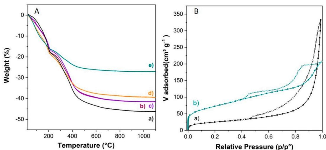
**Figure 4.** (A) TGA curves of [MgAl/TiO<sub>2</sub>] nanocomposites obtained by coprecipitation for different MgAl/TiO<sub>2</sub> ratios: (a) [Mg<sub>2</sub>Al-CO<sub>3</sub>], (b) [MgAl/TiO<sub>2</sub>]<sub>8</sub>, (c) [MgAl/TiO<sub>2</sub>]<sub>4</sub>, (d) [MgAl/TiO<sub>2</sub>]<sub>2</sub>, and (e) [MgAl/TiO<sub>2</sub>]<sub>0.66</sub>. (B) N<sub>2</sub> adsorption-desorption isotherms of (a) [Mg<sub>2</sub>Al-CO<sub>3</sub>] and (b) [MgAl/TiO<sub>2</sub>]<sub>0.66</sub>.
