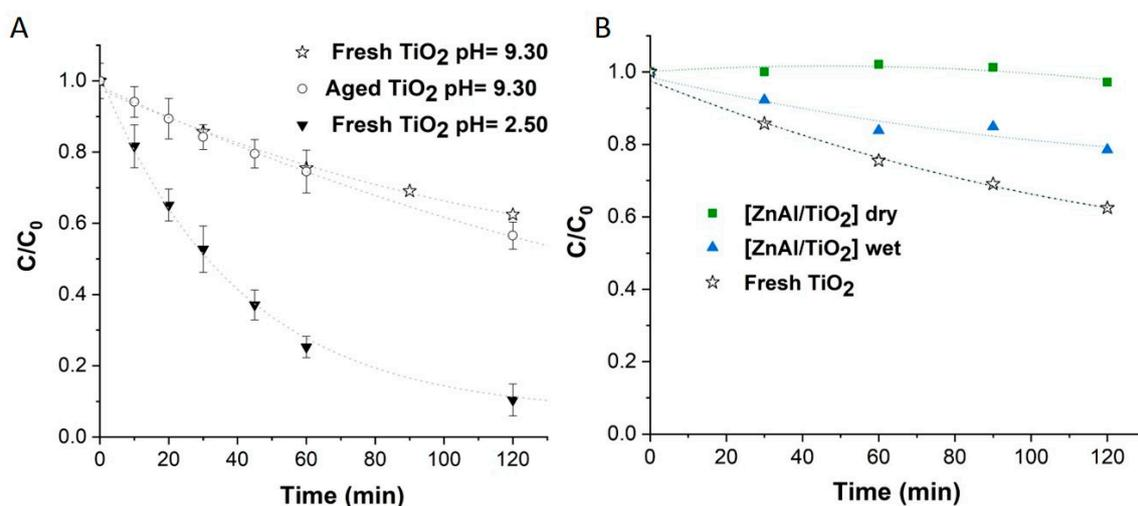
**Figure 6.** Variation of the concentration of OII at pH = 9.30 during photodegradation by (A) various colloidal TiO<sub>2</sub> dispersion and (B) [ZnAl-TiO<sub>2</sub>] nanocomposites prepared by impregnation. Conditions:  $[OII]_{initial} = 5.10^{-5}$  M;  $[TiO_2] = 0.5$  g L<sup>-1</sup> for all samples.
