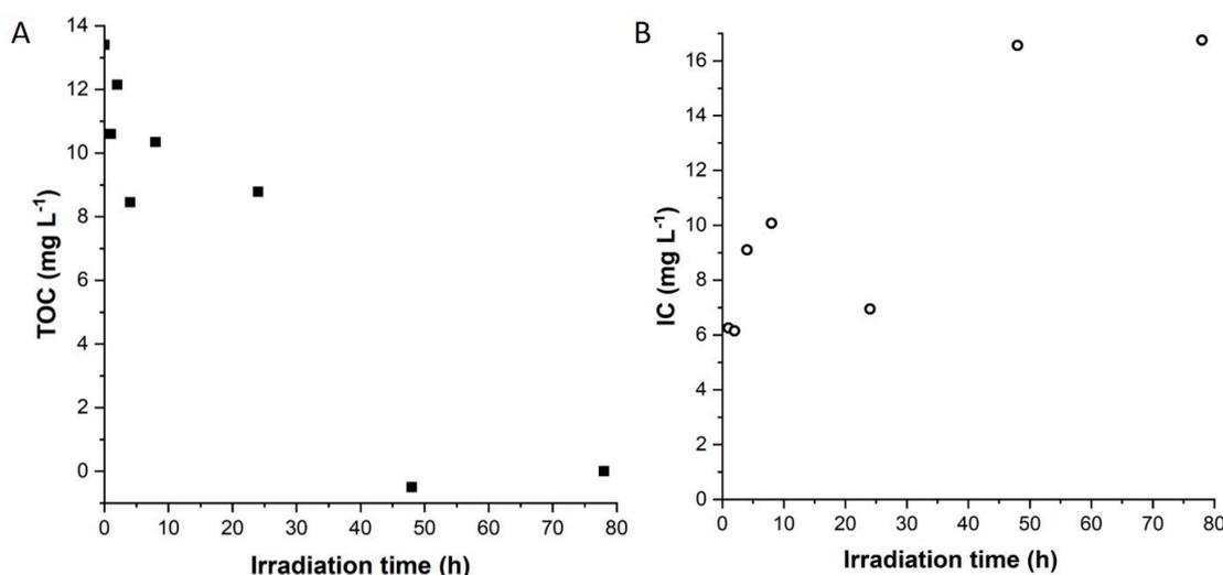
**Figure 8.** (A) Total organic carbon (TOC) and (B) inorganic carbon (IC) measurements under irradiation of OII in the presence of  $[\text{MgAl}/\text{TiO}_2]_{0.66}$ . Conditions:  $[\text{OII}] = 5.10^{-5}$  M,  $[\text{TiO}_2] = 0.5$  g L<sup>-1</sup>,  $m[\text{MgAl}/\text{TiO}_2]_{0.66} = 63.2$  mg L<sup>-1</sup>, pH = 9.30.
