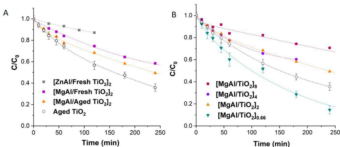
**Figure 7.** Variation of the concentration of OII at pH = 9.30 during photodegradation by nanocomposites prepared by direct coprecipitation (A) for ZnAl and MgAl LDH and fresh or aged  $TiO_2$  and (B) for different MgAl/ $TiO_2$  ratios.
