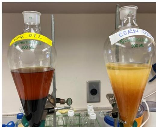
**Figure 1.** Difference between separation of glycerol from methyl ester of soybean oil (left) and corn oil (right).
