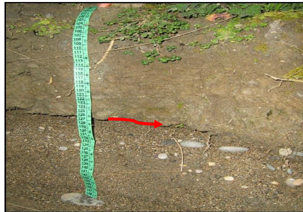
Figure 8. Transition of soil texture in a natural profile located near the site. Note the position of the red arrow where the soil texture transition takes place.
