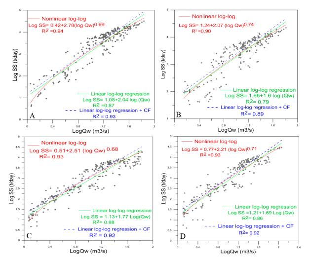
Figure 6. The developed rating curves (A) at station Duguda; (B) Maki; (C) Abura; and (D) Fite.
