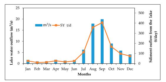
Figure 9. Suspended sediment concentration (SSC) and lake outlets.
