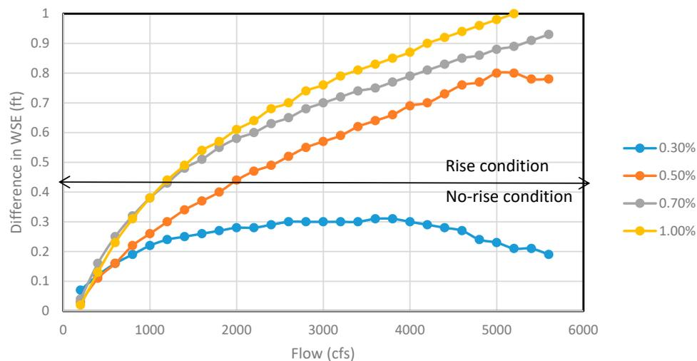
**Figure 5.** The difference in water surface elevation at most upstream before and after pier encasement (both rise and no-rise condition seen) for 20 ft channel section for different flows.
