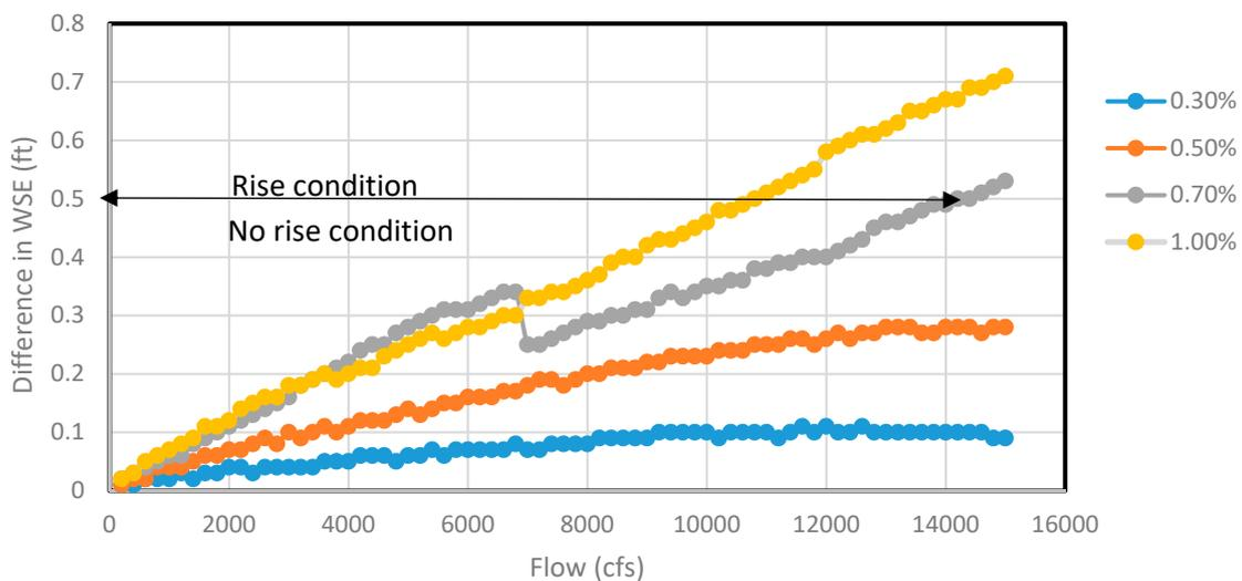
**Figure 8.** The difference in water surface elevation at immediate upstream before and after pier encasement (both rise and no-rise condition seen) for 100 ft channel section for different flows.
