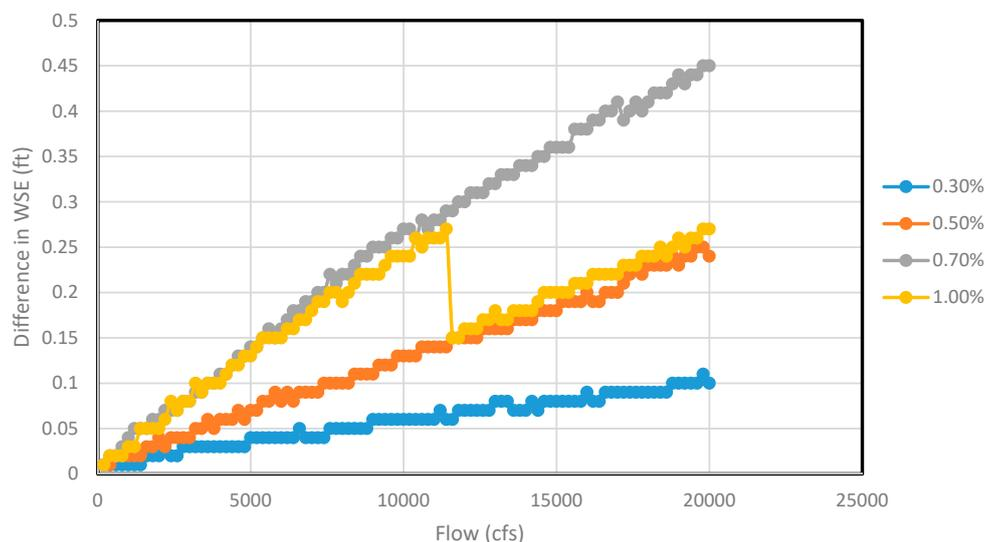
**Figure 10.** The difference in water surface elevation at immediate upstream before and after pier encasement (only no-rise condition seen) for 180 ft channel section for different flows.
