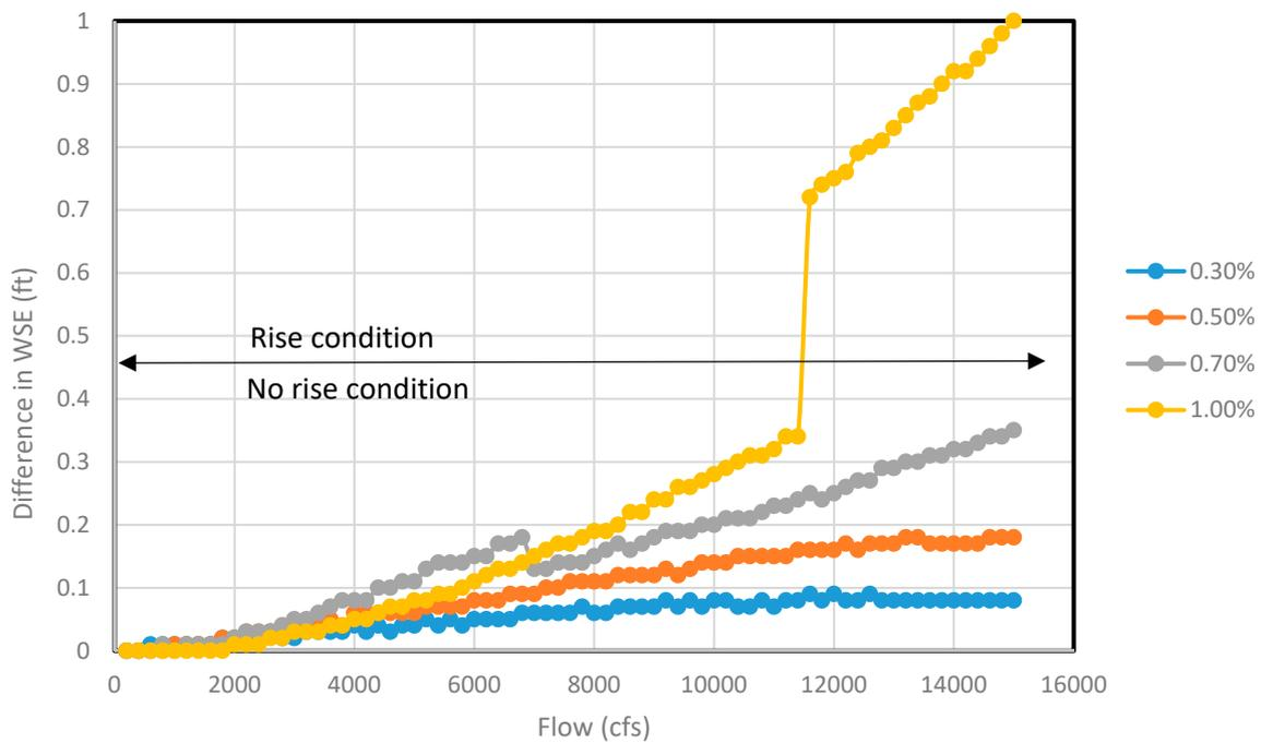
**Figure 7.** The difference in water surface elevation at most upstream before and after pier encasement (both rise and no-rise condition seen) for 100 ft channel section for different flows.
