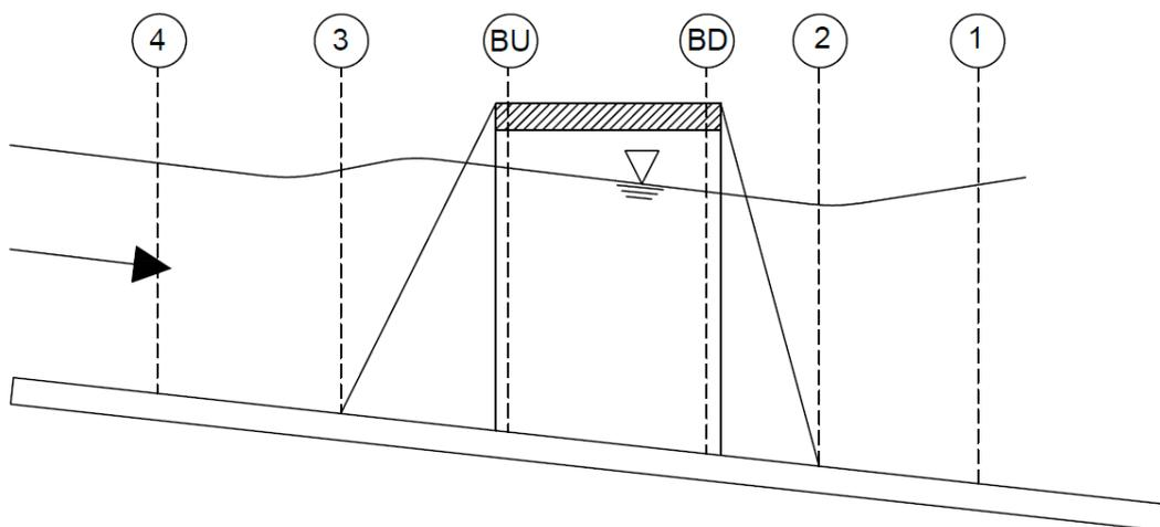
**Figure 2.** Channel profile and cross section locations.
