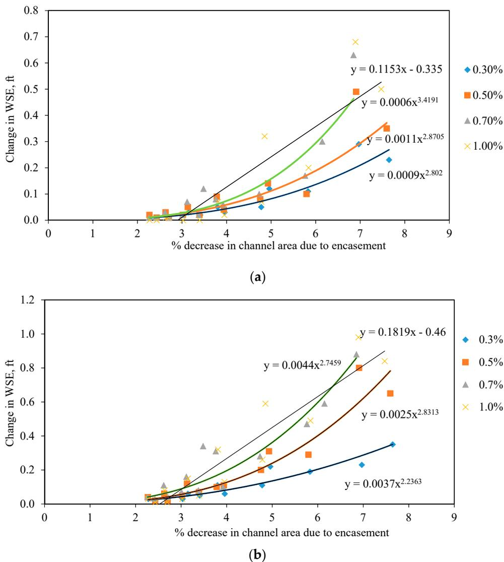
**Figure 11.** The difference in water surface elevation with respect to percentage change in area due to encasement for flow (a) 2400 cfs; (b) 5000 cfs.
