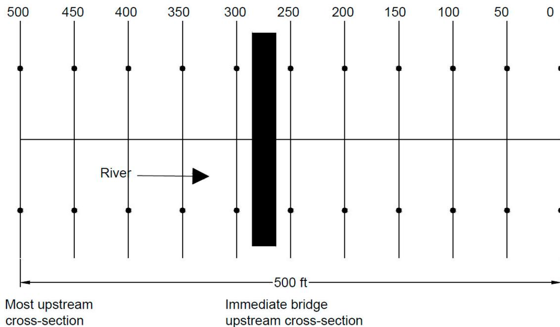
**Figure 3.** Channel cross-section in HEC-RAS with 180 ft bottom width.
