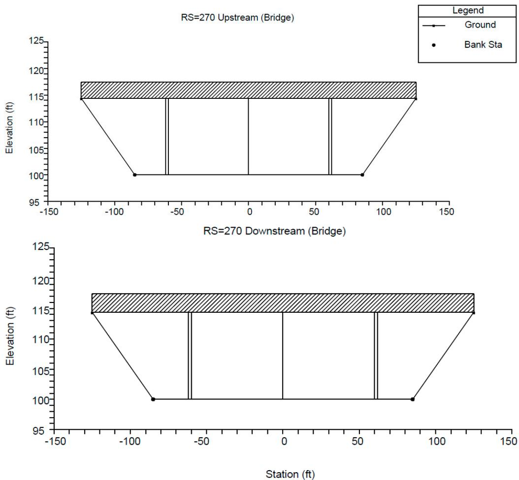
Figure 4. Bridge cross-section with pier location in the channel with 180 ft bottom width.
