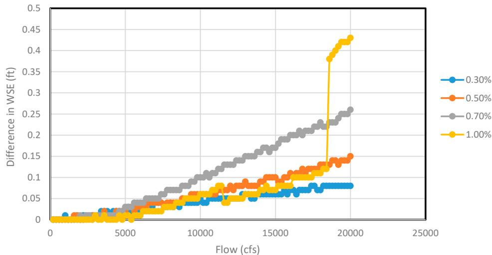
**Figure 9.** The difference in water surface elevation at most upstream before and after pier encasement (only no-rise condition seen) for 180 ft channel section for different flows.
