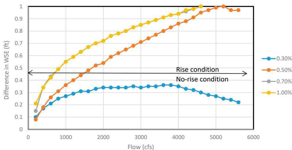
**Figure 6.** The difference in water surface elevation at immediate upstream before and after pier encasement (both rise and no-rise condition seen) for 20 ft channel section for different flows.
