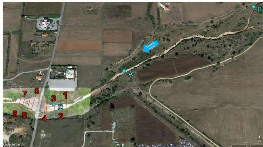
**Figure 2.** The eight cross-sections (red lines) and three erosion pins plots (blue dots) as located on studied reach of Kallifitos torrent, Drama, Greece. Between cross-sections 4 and 5 is an Irish bridge. The light color area indicates the area that was captured by the drone during the six flights.
