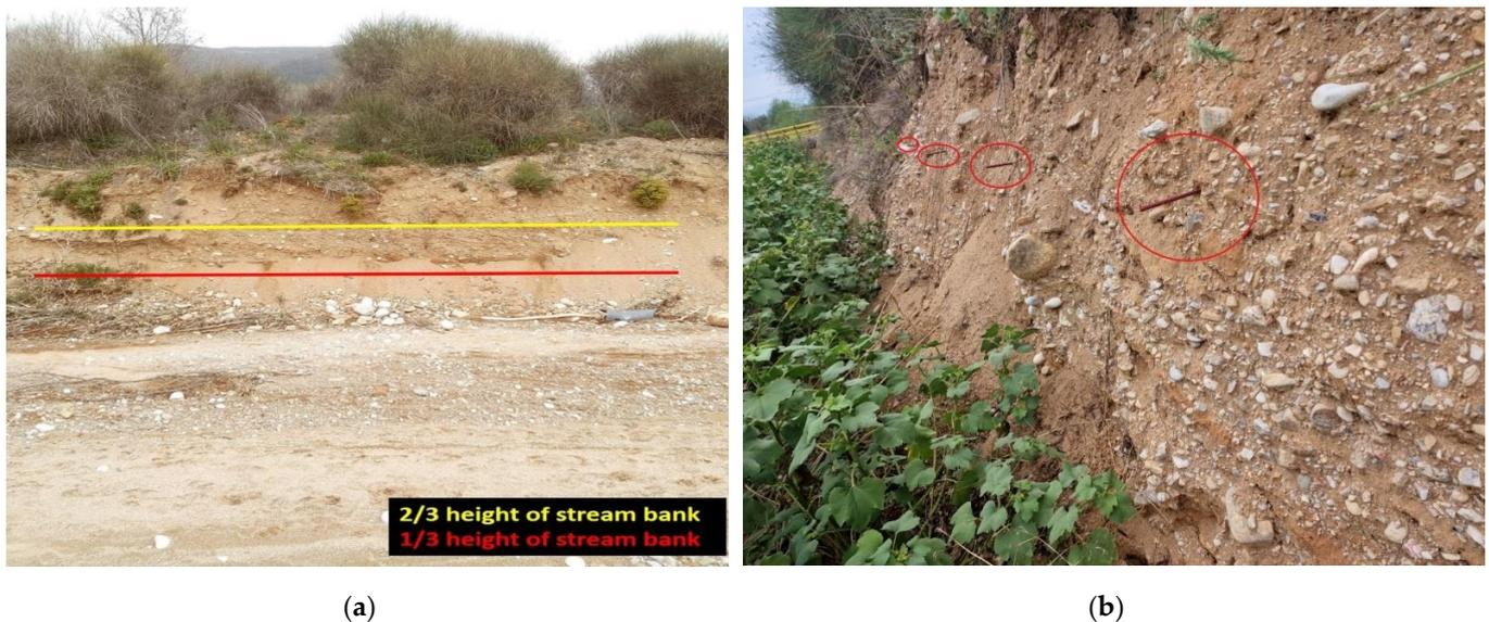
**Figure 4.** (a) A representative stream bank of the Kallifitos torrent with the upper erosion pins (2/3) in the yellow line and the lower erosion pins in the red line; (b) a representative stream bank of the Kallifitos torrent with erosion pins (red circles) installed at the upper part (2/3) while the lower part (1/3) was covered by soil deposition.
