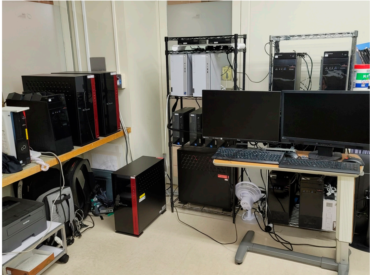
Figure S1. Custom-made consumer-type parallel computing cluster or “3C cluster”. The SVM cross-validation was performed using the EMG dataset of 19 acute stroke patients with various grades of upper extremity paresis specified.
