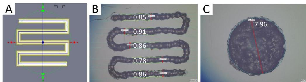
**Figure 2.** GelMA/OMA printability. A three-line print was designed in TSIM (A) which produced the lines shown (B) and the disc (C) using the settings in Table 1. All measurements are in mm. Scale bar 1mm.
