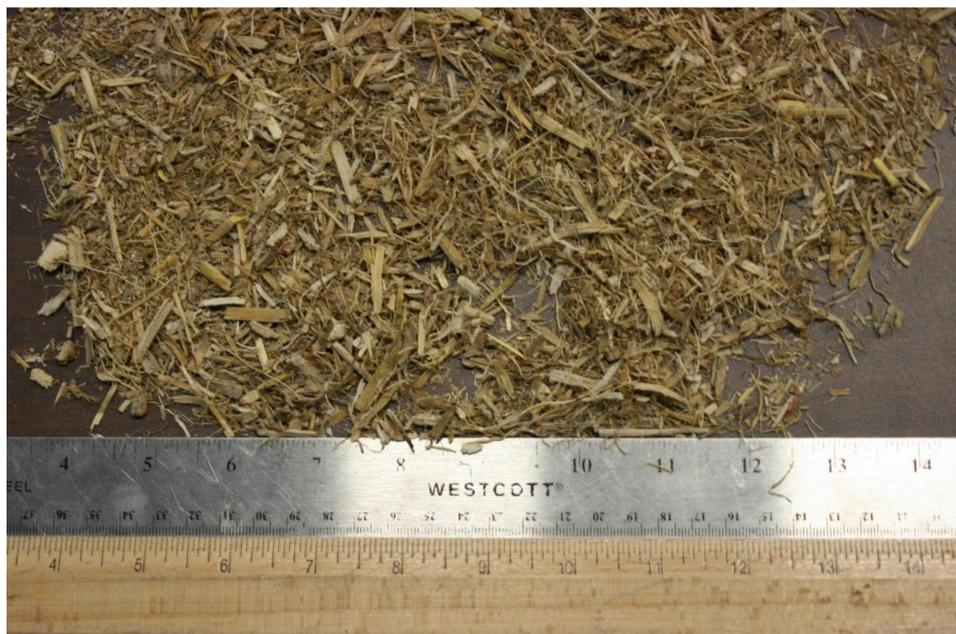
**Figure 2.** The corn stover after Stage-1 grinding.
