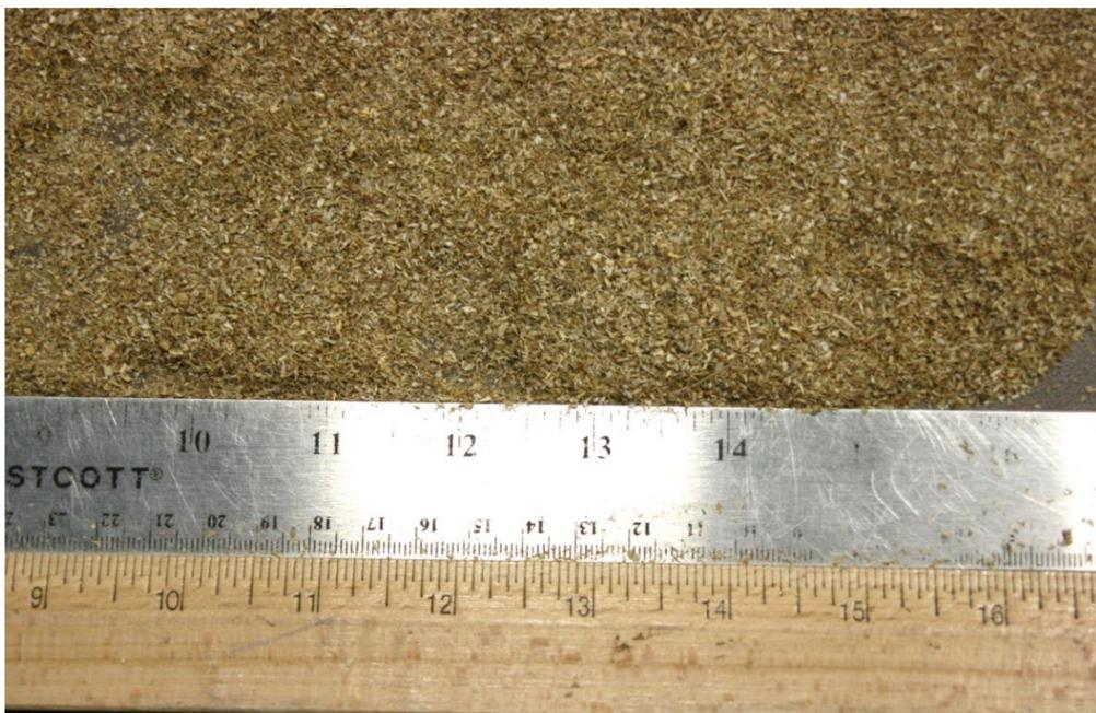
**Figure 6.** The corn stover after passing through the Wiley mill.
