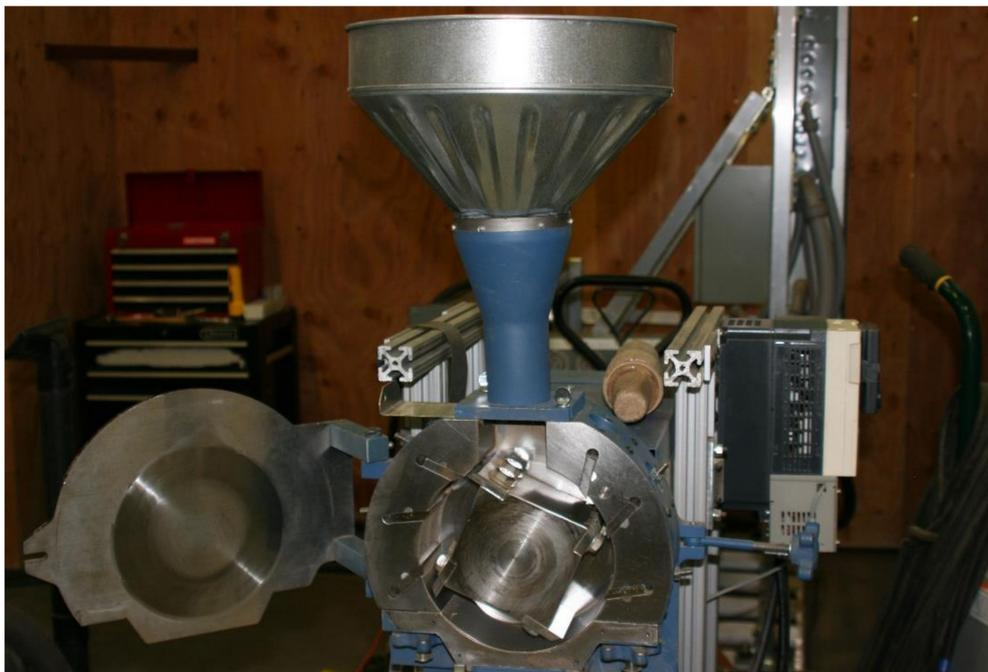
**Figure 4.** The laboratory scale Wiley mill with blades exposed.
