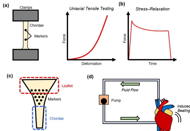
**Figure 4.** Mechanical characterizations of the atrioventricular heart valve (AHV) chordae tendineae through: (a) uniaxial mechanical testing, (b) stress-relaxation testing, (c) chordae-leaflet insertion region deformation tracking, and (d) an in vitro heart simulating flow loop.
