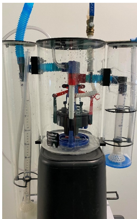
Figure S8. Picture of the BubbleVent prototype used for the study. The three water tanks enabled individual control of PIP, PEEP, T_i , and T_E .
