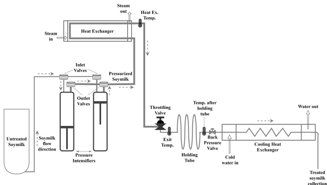
**Figure 1.** Ultra high pressure homogenization diagram.
