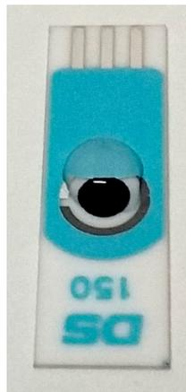
**Figure 4.** Direct contact between the cell suspension of pAb76-membrane-engineered Vero cells and the screen-printed working electrode.
