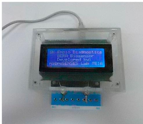
**Figure 5.** The handheld TCA screener with the disposable eight-channel electrode strip attached to the main measuring unit.
