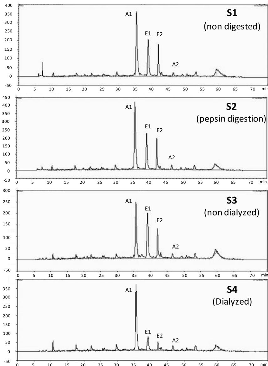
**Figure 1.** HPLC Chromatogram of the digested blackberry juice polyphenols. A1: cyanidin-3-glucoside, A2: cyanidin-3-malonyl glucoside, E1: lambertianin C, E2: sanguin H-6. (Corresponding tentative identification of peaks according to Mertz et al. [7]).
