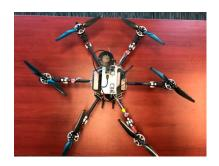
Figure 1. Tarot-RC 690 Hexacopter Unmanned Aerial System (UAS).
