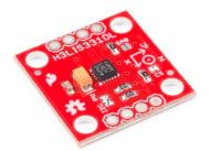
Figure 10. ST H3LIS331DL three-axis accelerometer.
