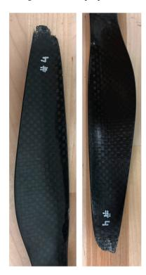
Figure 9. Broken propeller #4.
