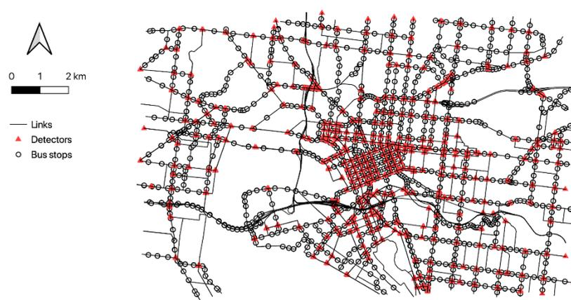
**Figure 4.** The spatial distribution of bus stops and detectors across the network.
