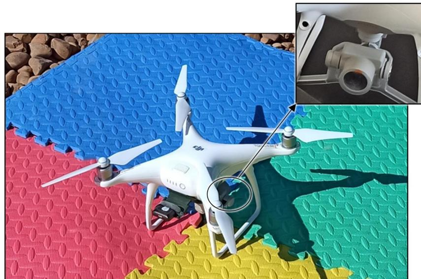
**Figure 5.** UAV DJI Phantom Advance quadcopter and detail of the DJI FC6310 RGB camera.
