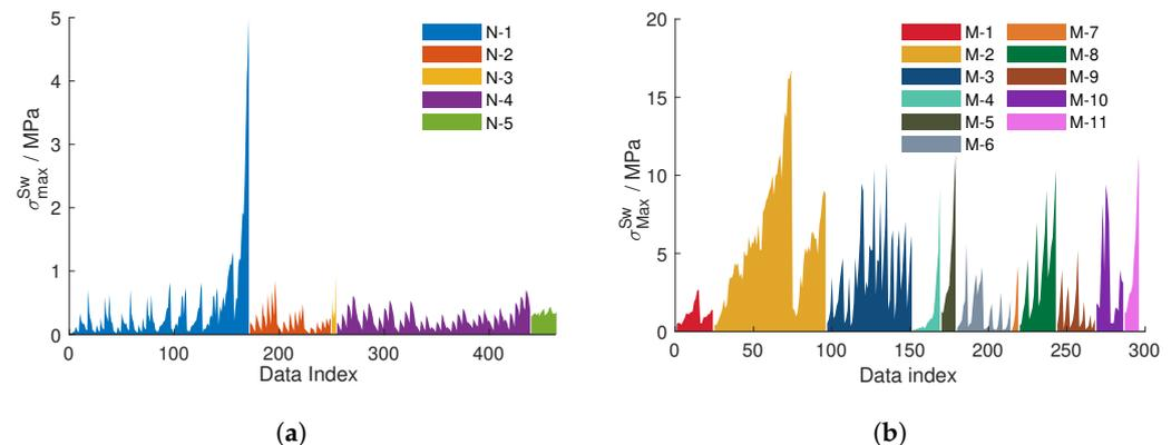
**Figure 3.** Distribution of maximum swelling pressure of (a) natural clay and (b) bentonite for each group within the dataset.
