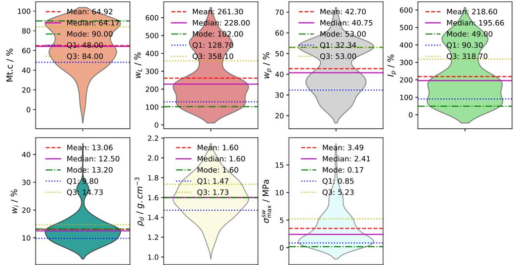
Figure 2. Statistical distribution of maximum swelling pressure of bentonite and other relevant properties.
