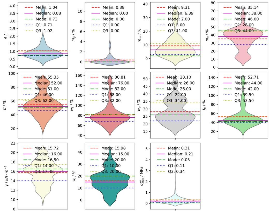
Figure 1. Statistical distribution of maximum swelling pressure of natural clay and other relevant properties.
