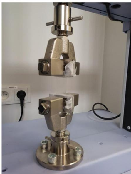
**Figure 4.** Attachments for the tensile strength study with the film mounted between the clamps.
