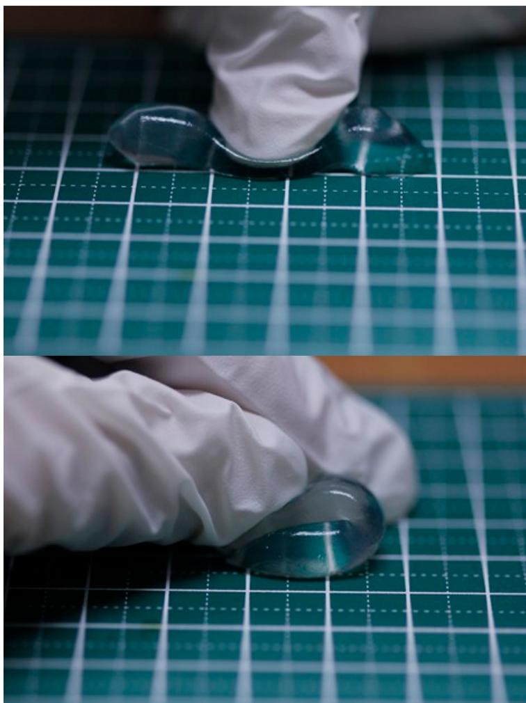
**Figure 2.** Pictures of a 5 wt % clay/1 wt % PAAS3500K/0.5 wt % TSPP blend hydrogel. A pressed gel (**top**) and a bent gel (**bottom**).
