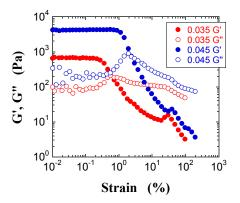
**Figure 9.** Double-logarithmic plots of *G*<sup>'</sup> (filled circles) and *G*<sup>"</sup> (open circles) for the PS suspensions at  $\varphi = 0.035$  (red) and 0.045 (blue) as a function of strain.
