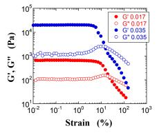
**Figure 8.** Double-logarithmic plots of the storage modulus (G', filled circles) and the loss modulus (G'', open squares) for the FS suspensions at  $\varphi = 0.017$  (red) and 0.035 (blue) as a function of strain.
