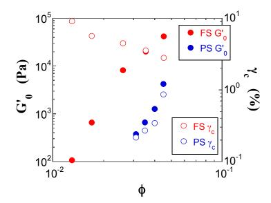
**Figure 10.** Double-logarithmic plots of the G' value in the linear region ( $G'_0$ , filled circles) and the critical oscillatory shear strain ( $\gamma_c$ , open circles) for the FS (red) and PS (blue) suspensions as a function of  $\varphi$ .
