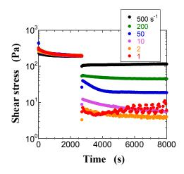
**Figure 3.** Plots of the transient shear stress for the FS suspension at  $\varphi = 0.017$  at the shear rates of 1 s<sup>-1</sup> (filled red circle), 2 s<sup>-1</sup> (filled orange circle), 10 s<sup>-1</sup> (filled purple circle), 50 s<sup>-1</sup> (filled blue circle), 200 s<sup>-1</sup> (filled green circle), and 500 s<sup>-1</sup> (filled black circle) as a function of time.
