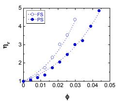
**Figure 7.** The relative viscosity values of the FS (open blue circle) and PS suspensions (filled blue circle) at the shear rate of  $10^3 \text{ s}^{-1}$  as a function of  $\varphi$ . The dashed lines represent fit to the Krieger and Dougherty equation.
