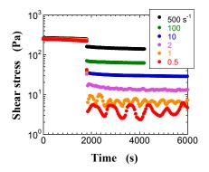
**Figure 4.** Plots of the transient shear stress for the precipitated silica (PS) suspension at  $\varphi = 0.030$  at the shear rates of 0.5 s<sup>-1</sup> (filled red circle), 1 s<sup>-1</sup> (filled orange circle), 2 s<sup>-1</sup> (filled purple circle), 10 s<sup>-1</sup> (filled blue circle), 100 s<sup>-1</sup> (filled green circle), and 500 s<sup>-1</sup> (filled black circle) as a function of time.
