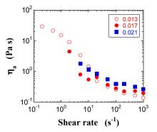
**Figure 5.** Double-logarithmic plots of the apparent steady-state shear viscosities ( $\eta_a$ ) for the FS suspensions at  $\varphi = 0.013$  (open red circle), 0.017 (filled red circle), and 0.021 (filled blue square) as a function of the shear rate.
