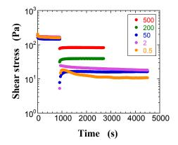
**Figure 2.** Plots of the transient shear stress for the FS suspension at the volume fraction of silica  $\varphi = 0.013$  at the shear rates of  $0.5 \text{ s}^{-1}$  (filled orange circle),  $2 \text{ s}^{-1}$  (filled purple circle),  $50 \text{ s}^{-1}$  (filled blue circle),  $200 \text{ s}^{-1}$  (filled green circle), and  $500 \text{ s}^{-1}$  (filled red circle) as a function of time.
