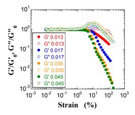
**Figure 11.** Double-logarithmic plots of  $G'/G'_0$  (filled circles) and  $G''/G''_0$  (open circles) for the FS suspensions at  $\varphi = 0.013$  (red), 0.017 (red), 0.035 (orange), and 0.045 (green) as a function of strain.  $G''_0$  is the loss modulus in the linear region.
