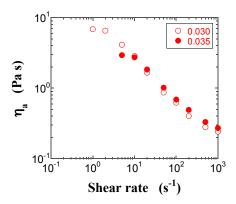
**Figure 6.** Double-logarithmic plots of the apparent steady-state shear viscosities for the PS suspensions at  $\varphi = 0.030$  (open red circle) and 0.035 (filled red circle) as a function of the shear rate.
