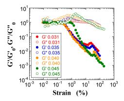
**Figure 12.** Double-logarithmic plots of  $G'/G'_0$  (filled circles) and  $G''/G''_0$  (open circles) for the PS suspensions at  $\varphi = 0.031$  (red), 0.035 (red), 0.040 (orange), and 0.045 (green) as a function of strain.
