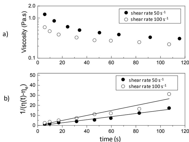
**Figure 1.** (a) Typical thixotropic behavior of a rheological time dependent gel after the application of constant shear rates of 50 1/s and 100 1/s; (b) schematic of the approach used to determine the parameters defining the structural parameter  $\lambda(\dot{\gamma}, t)$  from Equation (10). Data used are from a 5% silica gel.
