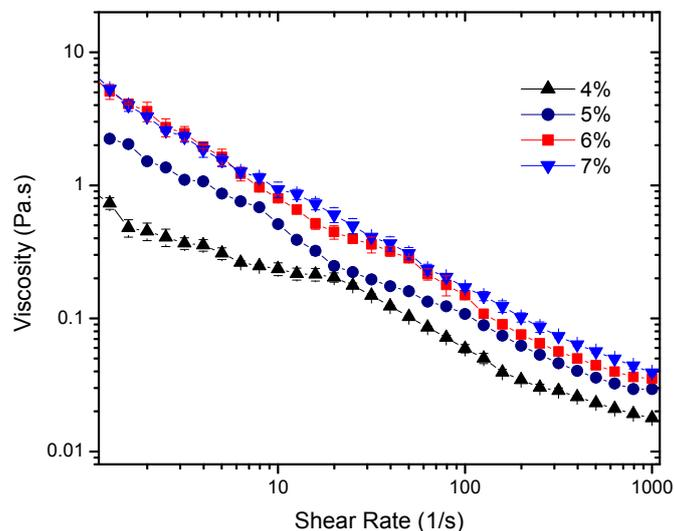
**Figure 3.** Viscosity (mean) as a function of shear rate for 4%, 5%, 6%, and 7% gels. These curves describe the flow behavior of the sheared and time independent fluid. The Extended Herschel-Bulkley model was applied to describe the flow characteristics of the gels. Measurements were carried out in triplicate. Error bars shown in the plot were calculated using a 95% confidence interval determined with the software OriginPro 2016 (OriginLab Corporation, Northampton, MA, USA).
