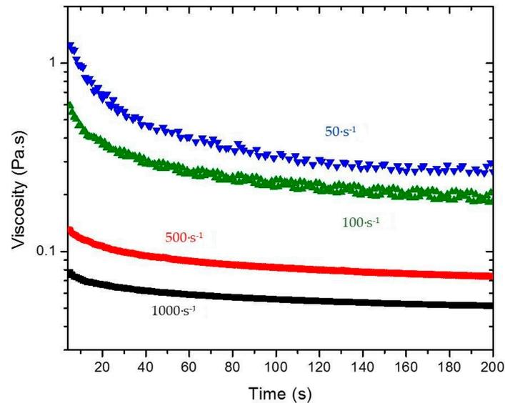
**Figure 6.** Viscosity of 4% “intact” gel as a function of time at different constant shear rates (50, 100, 500, and 1000  $s^{-1}$ ).
