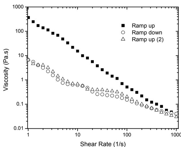
**Figure 2.** Viscosity measurements of 6% gel. Three runs were carried out using the same sample: shear rate was increased from 1 to  $1000 \text{ s}^{-1}$  (ramp up), varied from  $1000$  to  $1 \text{ s}^{-1}$  (ramp down), and increased from 1 to  $1000 \text{ s}^{-1}$  (ramp up 2).
