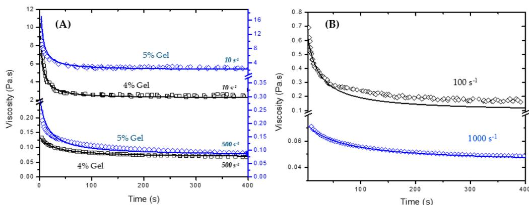
**Figure 7.** (A) Experimental (symbols) and predicted viscosity (lines) data for 4% and 5% gels at 10 and 500 s<sup>-1</sup>. The 4% data is plotted in the left Y-axis and is represented by square symbols. The 5% data is plotted in the right Y-axis and is represented by diamond symbols; (B) calculated viscosity assuming  $\lambda_e = 1$  for 4% gels at shear rates of 100 and 1000 s<sup>-1</sup>.
