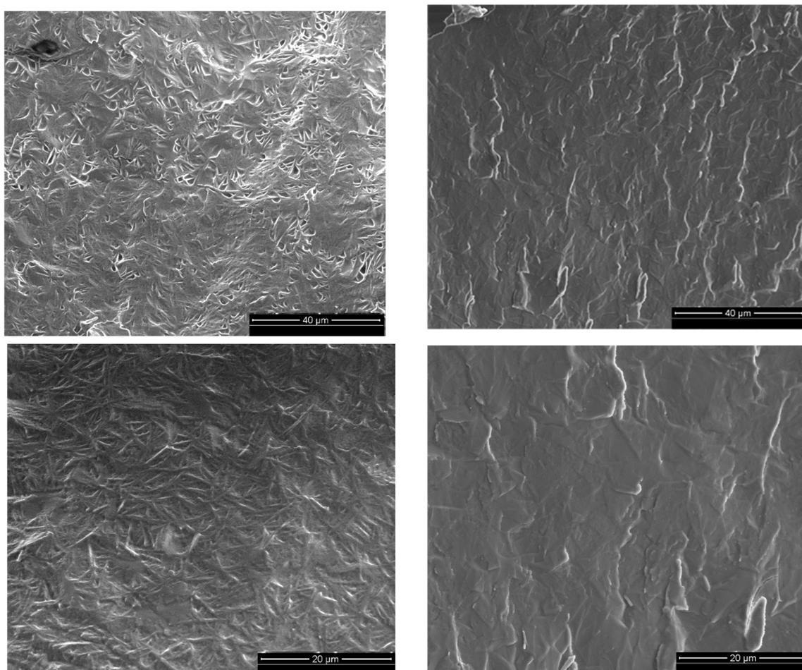
**Figure 5.** Cryo-SEM micrographs of 6% “intact” (on the left) and pre-sheared gels (on the right). Micrographs at different magnifications: 40 and 20  $\mu\text{m}$  (from top to the bottom).
