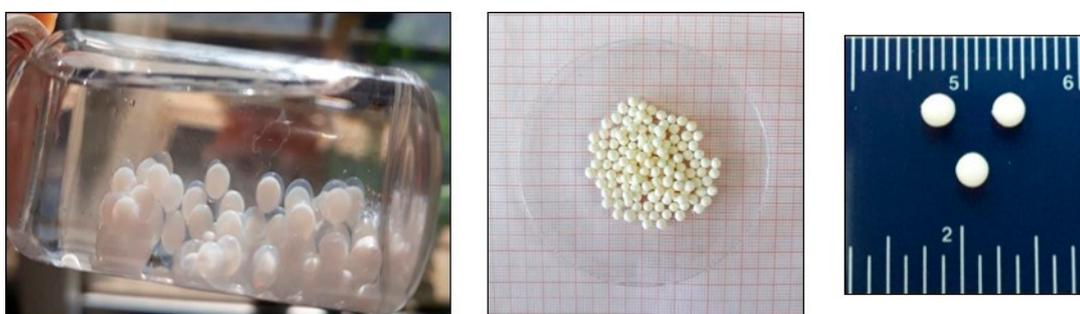
**Figure 1.** Spherical polyurea (PUA) aerogel beads during solvent exchange with acetone (left) and after dried with supercritical fluid (SCF) CO<sub>2</sub> (middle and right).
