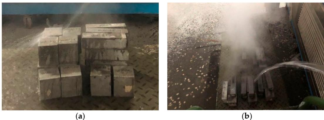
**Figure 1.** Cooling of specimens after high-temperature exposure. (a) 200 °C and (b) 600 °C.
