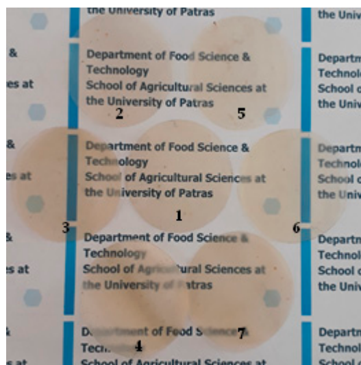
Figure 5. Photo images (1) pure CS/PVOH films, (2) CS/PVOH/5HNT, (3) CS/PVOH/10HNT, (4) CS/PVOH/15HNT, (5) CS/PVOH/5TO@HNT, (6) CS/PVOH/10TO@HNT, and (7) CS/PVOH/5TO@HNT films.
