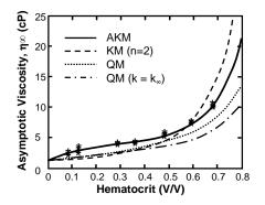
**Figure 2.** Comparison of regression of asymptotic viscosity vs. hematocrit with the Asymptotic Krieger model (AKM), Krieger model (n = 2), the Quemada model, and the asymptotic Quemada model ( $k = k_{\infty}$ ) to the experimental data of Brooks et al. (asterisks) [49]. (Shear rate > 100 s<sup>-1</sup>).
