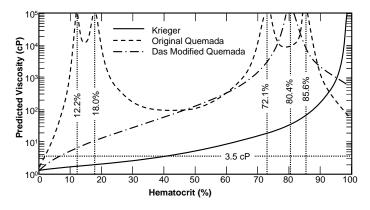
**Figure 1.** The zero-shear viscosity prediction of the original Quemada model, the modified Quemada model, and the Krieger model with n = 2. Discontinuities and regions where the viscosity is inversely proportional to hematocrit were found for both forms of the Quemada model.
