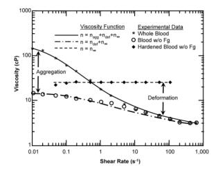
**Figure 4.** Contribution of aggregation and cell deformation on viscosity for canine red blood cells (RBCs) at a hematocrit of 45% and a temperature of 37 °C. The lines for each case are generated from the modified Krieger model with the appropriate optimal parameters. Experimental data from Chien [50].
