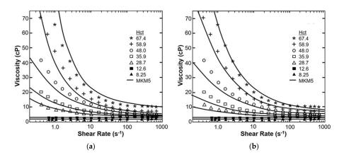
**Figure 3.** A comparison of shear thinning according to the MKM5 (**a**) and the Quemada model (**b**) vs. the experimental data of Brooks et al. [49] (symbols) for seven values of hematocrit and spanning four decades of shear rate.
