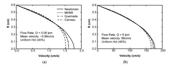
**Figure 6.** The fully-developed, steady-state velocity profile for Poiseuille flow of 40% hematocrit blood in a tube. Results compare the Newtonian solution (Parabolic), with the Modified Krieger model, the modified Quemada Model, and the model used by Jung et al. at a flow rate of 0.06 lpm (**a**) and 6 lpm (**b**).
