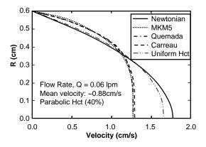
**Figure 7.** Comparison of the fully-developed, steady-state velocity profile for Poiseuille flow of blood assuming a parabolic hematocrit profile vs. a uniform profile. The results of the MKM5 model and Quemada model overlap.
