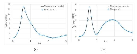
**Figure 3.** Horizontal-exciting forces on a bottom fixed cylindrical body placed in front of an orthogonal breakwater using the method of images: (**a**) horizontal-exciting force on *x*-axis; (**b**) horizontal-exciting force on *y*-axis.
