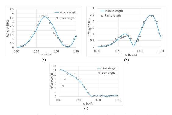
**Figure 13.** Exciting forces on a floating cylindrical floater placed in front of an orthogonal breakwater of finite length: (a) horizontal-exciting force on *x*-axis; (b) horizontal-exciting force on *y*-axis; (c) vertical-exciting force on *z*-axis. The results are compared with the corresponding values of the same floater placed in front of an infinite length orthogonal breakwater.
