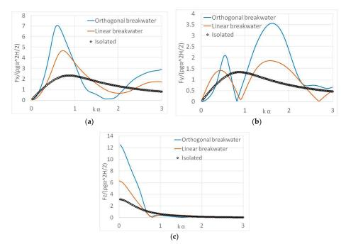
**Figure 11.** Exciting forces on a floating cylindrical floater placed in front of a linear breakwater using the method of images: (a) horizontal-exciting force on *x*-axis; (b) horizontal-exciting force on *y*-axis; (c) vertical-exciting force on *z*-axis. The results are compared with the corresponding values of the same floater placed in front of a right-angle-shaped breakwater and in isolation condition (i.e., without the presence of the breakwater).
