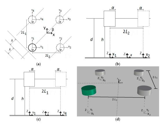
**Figure 2.** 2-D and 3-D representation of the floaters in the image method: (**a**) plan view in 2-D; (**b**) side view -xz in 2-D; (**c**) side view -yz in 2-D. The image devices are denoted dashed; (**d**) side view -xyz in 3-D. The image devices are depicted in gray color. The dashed lines in black denote the location of the orthogonal breakwater.
