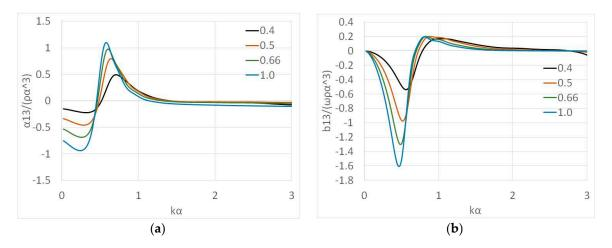
**Figure 9.** Hydrodynamic coefficients of a floating cylindrical floater placed in front of an orthogonally shaped breakwater using the method of images for a/h = 0.4; 0.5; 0.66; 1.0: (**a**) surge-added mass due to motion of the body in heave (**b**) surge damping coefficient due to motion of the body in heave.
