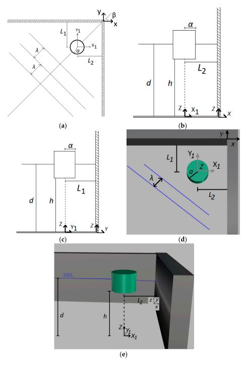
**Figure 1.** 2-D and 3-D representation of a vertical cylindrical floater in front of an orthogonal breakwater: (a) plan view in 2-D; (b) side view -xz in 2-D; (c) side view -yz in 2-D; (d) plan view -xyz in 3-D; (e) side view -xzy in 3-D.
