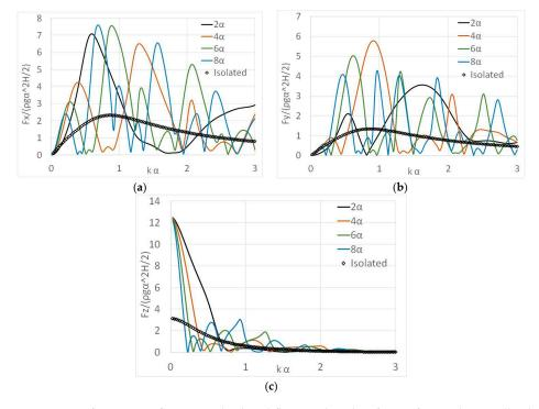
**Figure 4.** Exciting forces on a floating cylindrical floater placed in front of an orthogonally shaped (right angle) breakwater using the method of images for  $L_1 = L_2 = 2\alpha$ ,  $4\alpha$ ,  $6\alpha$ ,  $8\alpha$ : (a) horizontal-exciting force on *x*-axis; (b) horizontal-exciting force on *y*-axis; (c) vertical-exciting force on *z*-axis. The results are also compared with the corresponding values of the same isolated floater (i.e., without the presence of the walls).
