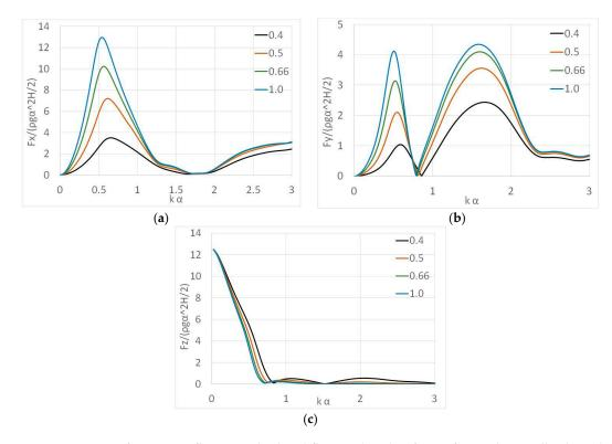
**Figure 7.** Exciting forces on a floating cylindrical floater placed in front of an orthogonally shaped (right angle) breakwater using the method of images for a/h = 0.4; 0.5; 0.66; 1.0: (**a**) Horizontal-exciting force on *x*-axis; (**b**) Horizontal-exciting force on *y*-axis; (**c**) Vertical-exciting force on *z*-axis.
