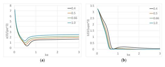
**Figure 8.** Hydrodynamic coefficients of a floating cylindrical floater placed in front of an orthogonally shaped (right angle) breakwater using the method of images for a/h = 0.4; 0.5; 0.66; 1.0: (**a**) heave added mass due to motion of the floater in heave (**b**) heave damping due to motion of the floater in heave.
