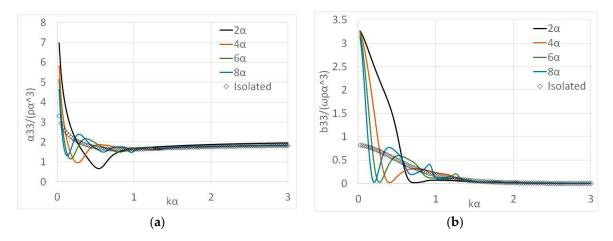
**Figure 5.** Hydrodynamic coefficients of a floating cylindrical floater placed in front of an orthogonally shaped (right angle) breakwater using the method of images for  $L_1 = L_2 = 2\alpha$ ,  $4\alpha$ ,  $6\alpha$ ,  $8\alpha$ : (**a**) heave added mass due to motion of the body in heave; (**b**) heave damping due to motion of the body in heave. The results are also compared with the corresponding values of the same isolated floater (i.e., without the presence of the walls).
