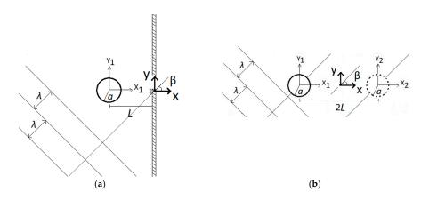
**Figure 10.** 2-D representation of a vertical cylindrical floater in front of a linear vertical breakwater: (a) plan view of the floater-breakwater system; (b) floaters' representation in the image method (the image device is denoted dashed).
