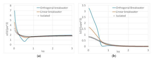
**Figure 12.** Hydrodynamic coefficients of a floating cylindrical floater placed in front of a linear breakwater using the method of images: (**a**) heave added mass due to motion of the floater in heave (**b**) heave damping coefficient due to motion of the floater in heave. The results are compared with the corresponding values of the same floater placed in front of an orthogonal breakwater and in isolation condition (i.e., without the presence of the breakwater).
