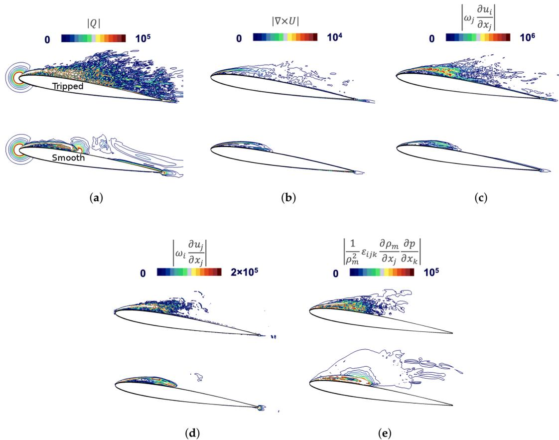
**Figure 11.** Distribution of vorticity properties for the smooth and tripped cases at  $Y = 0.5$ . (a) Magnitude of  $Q$ -criterion. (b) Magnitude of velocity curl. (c) Magnitude of stretching term. (d) Magnitude of dilatation term. (e) Magnitude of baroclinic term.
