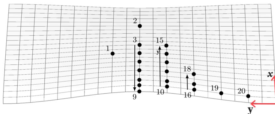
**Figure 1.** Location and numberings of the pressure probes used in the Delft twist11 foil tests [6].
