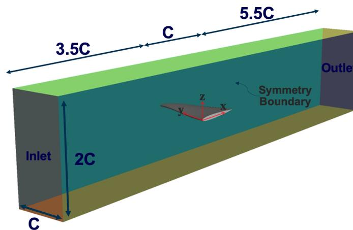
**Figure 2.** Computational domain employed in the current numerical simulations.
