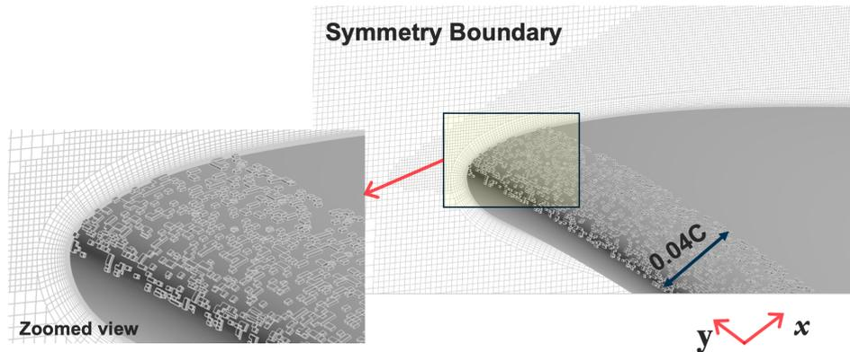
Figure 4. Roughness elements distribution in the leading edge of the foil.
